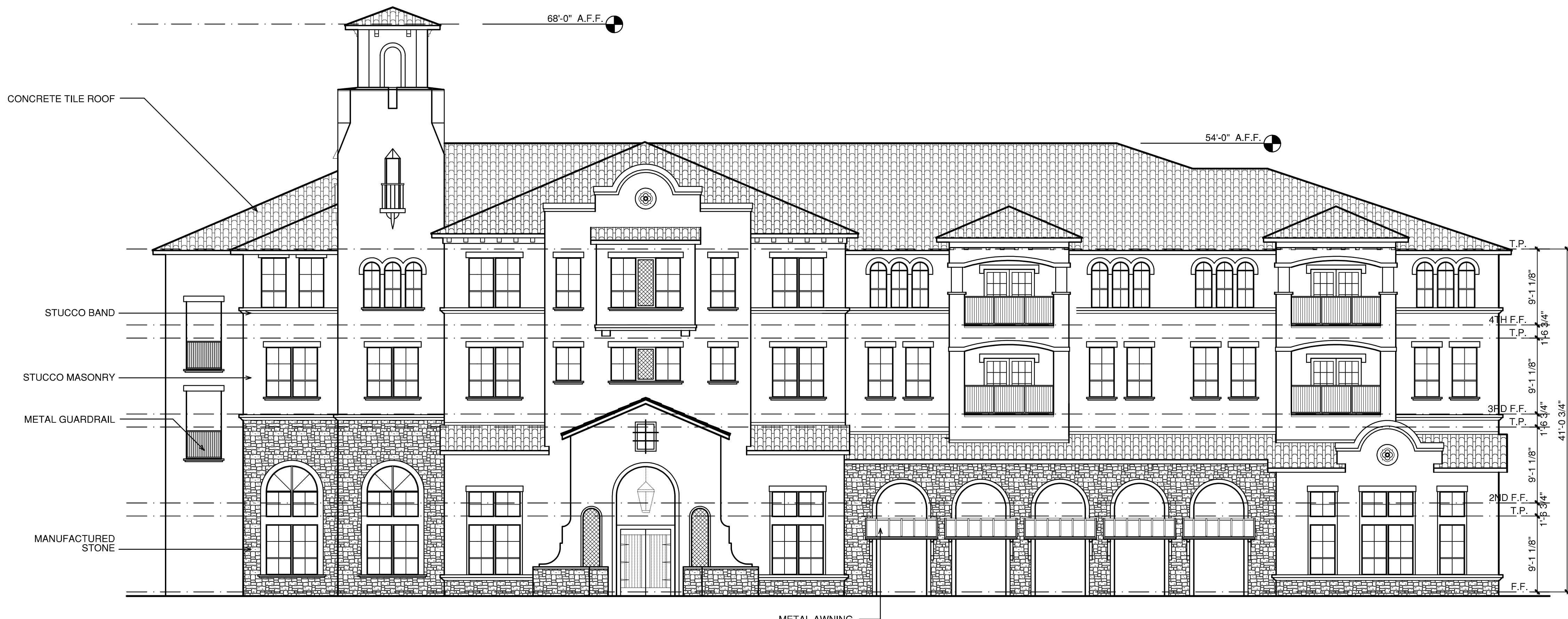
1 FRONT ELEVATION -ENTRY (TYPICAL 4 STORY) SCALE: 1/8"=1'-0"
