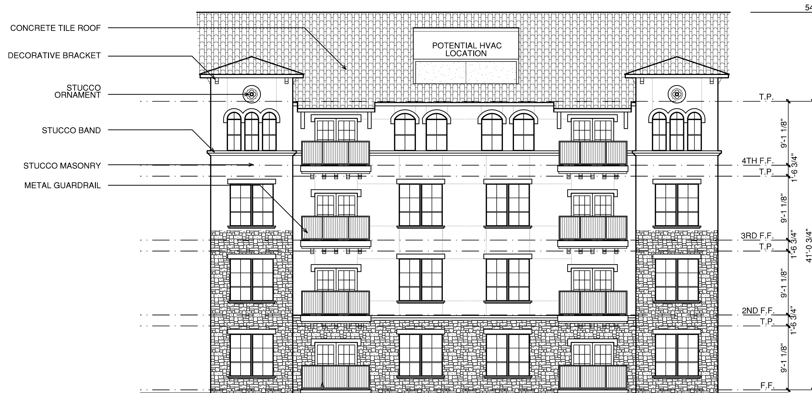
5 REAR ELEVATION - POOL SIDE (TYPICAL 4 STORY)
