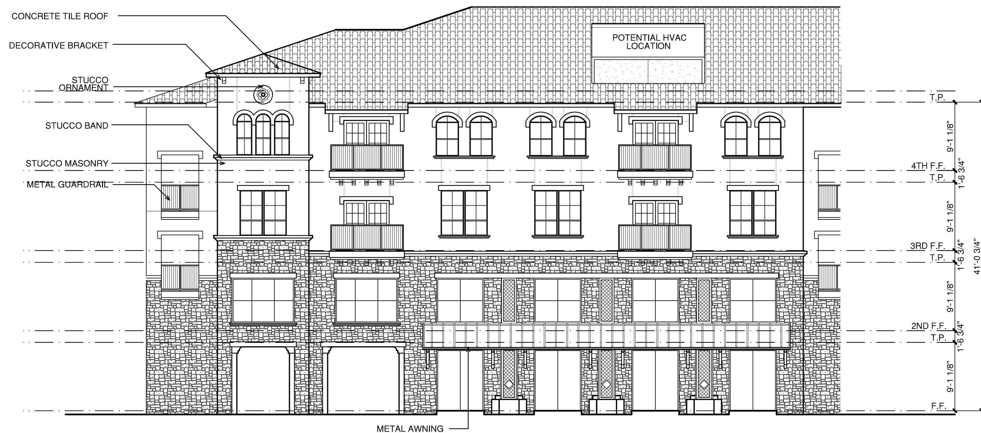
6 REAR ELEVATION - POOL SIDE (TYPICAL 4 STORY)
