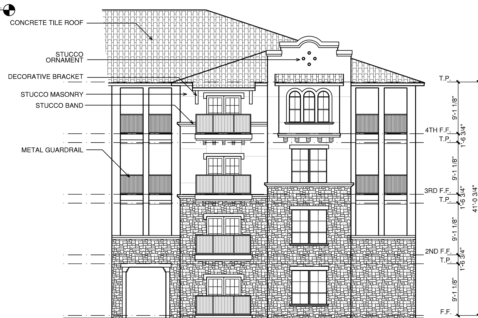
4 REAR ELEVATION - POOL SIDE (TYPICAL 4 STORY)
