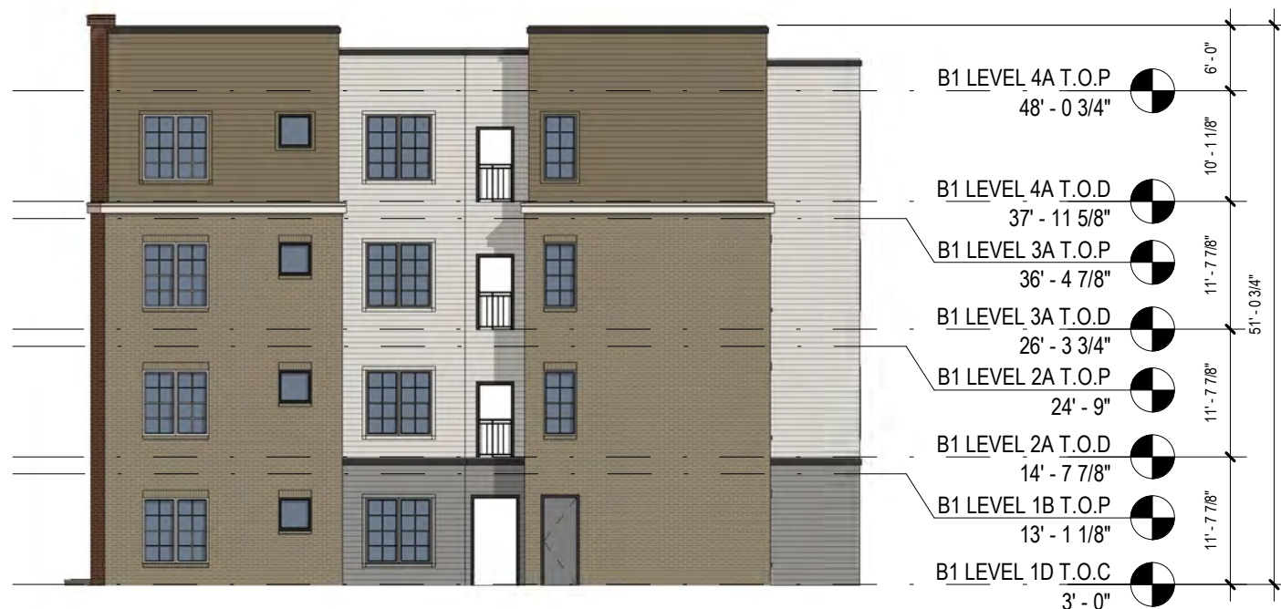
2 Building 1 - East Elevation - SUP Scale: 1/16" = 1'-0"
