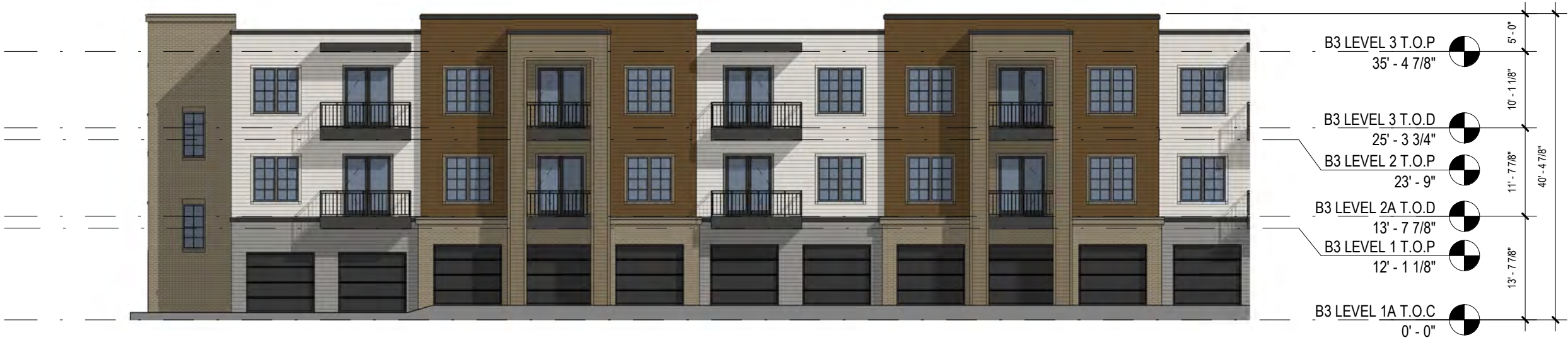
1 Building 4 - Courtyard North Elevation 02 - SUP Scale: 1/16" = 1'-0"
