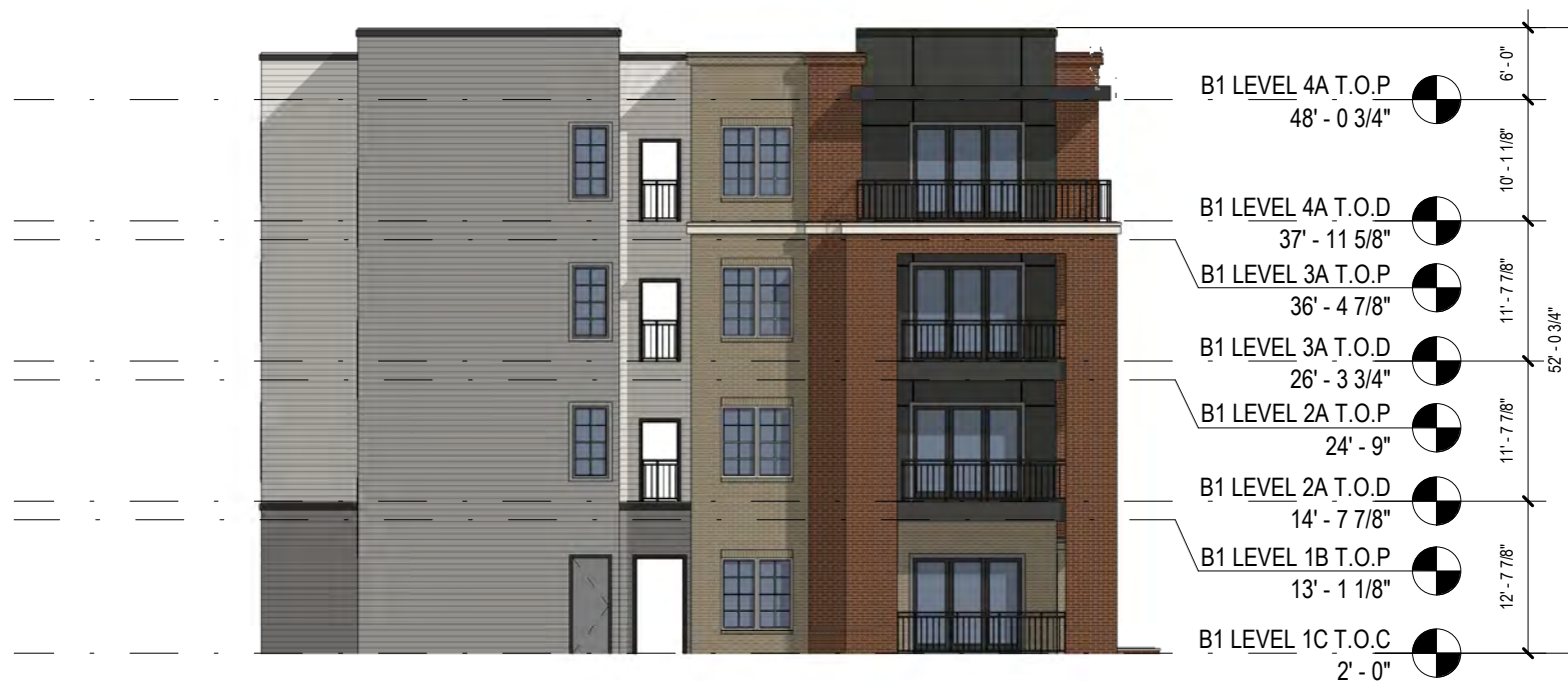
1 Building 1 - North Elevation - SUP Scale: 1/16" = 1'-0"
