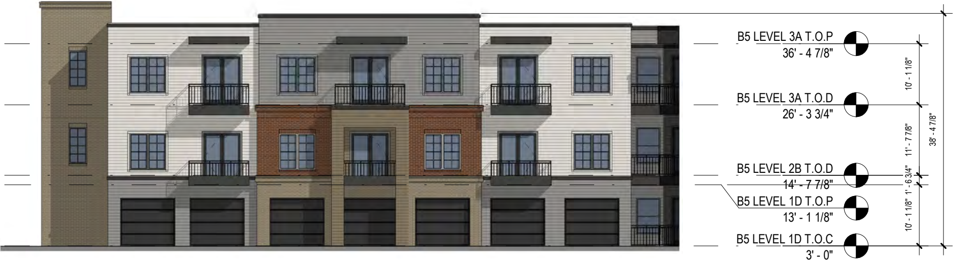
3 Building 5 - Courtyard West Elevation - SUP
