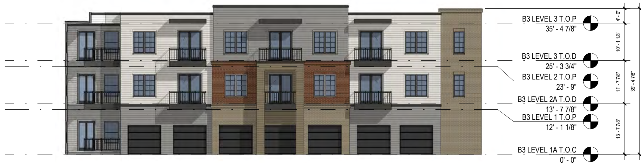
3 Building 4 - Courtyard West Elevation - SUP Scale: 1/16" = 1'-0"
