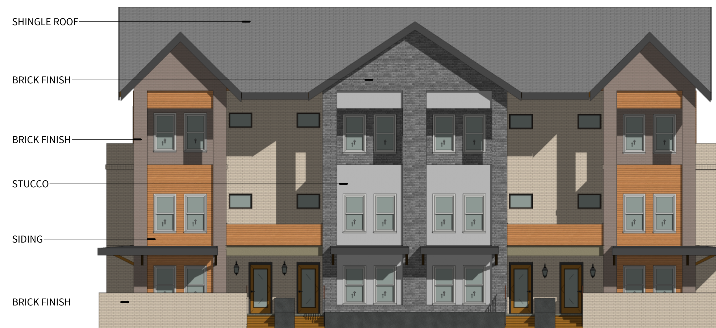
① NORTH ELEVATION - GREEN BUILDING TYPE SCALE: 1/8" = 1'-0"
