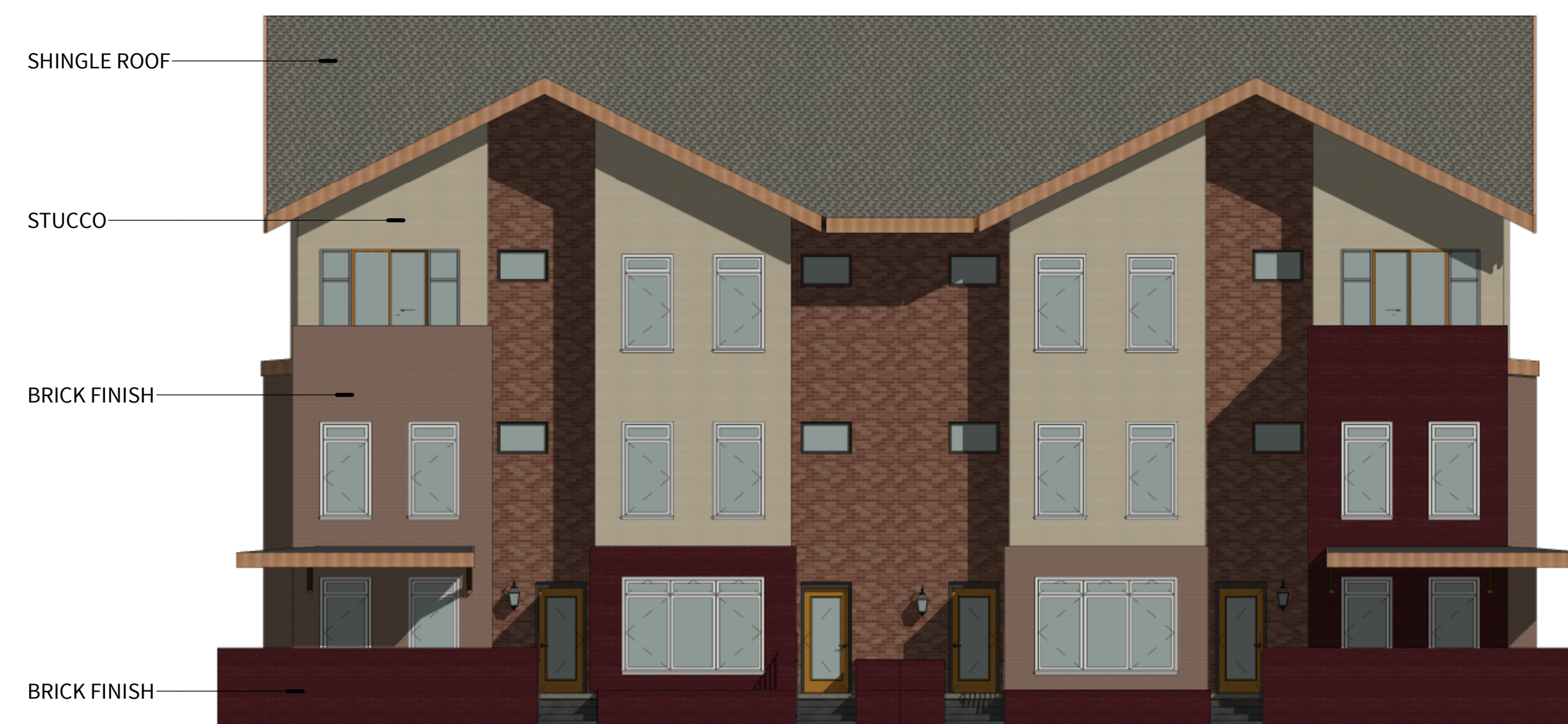
① NORTH ELEVATION - YELLOW BUILDING TYPE SCALE: 1/8" = 1'-0"
