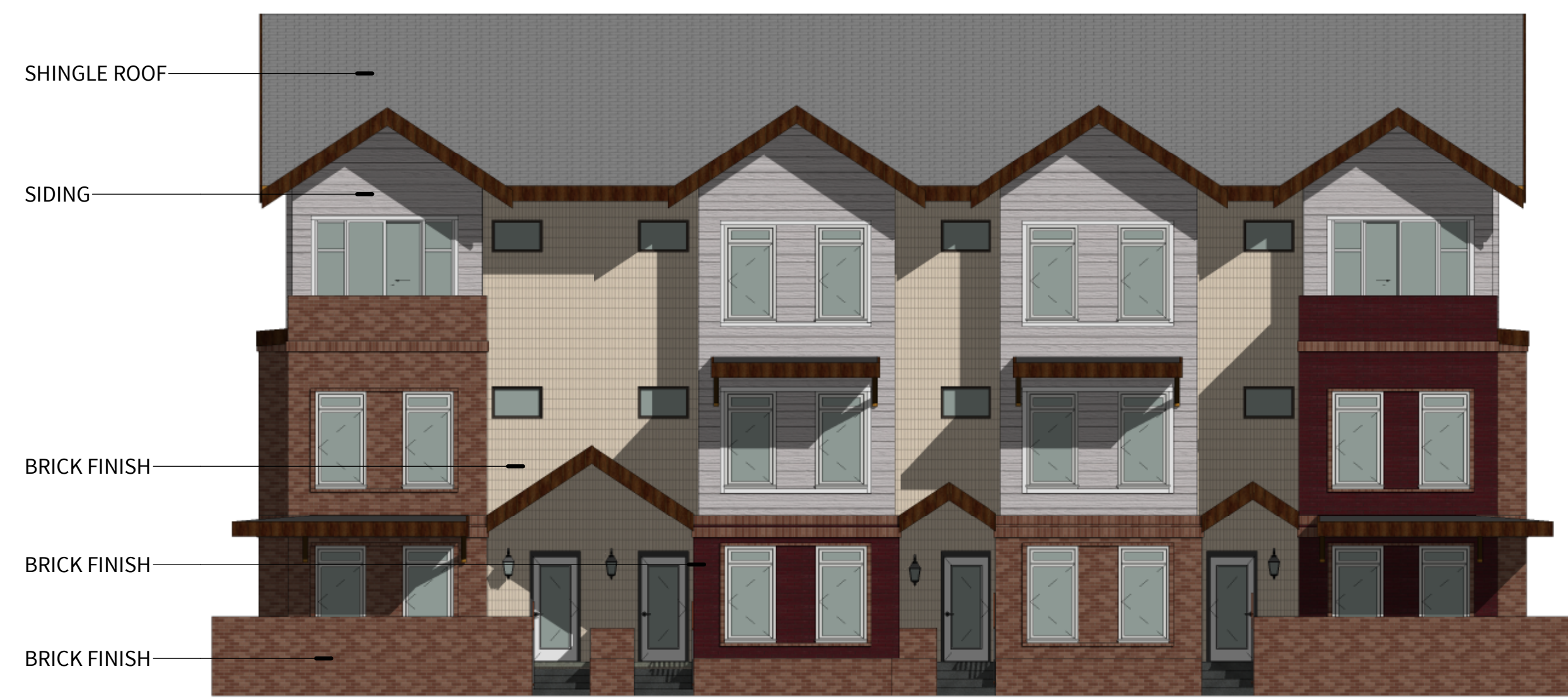
① NORTH ELEVATION - BLUE BUILDING TYPE SCALE: 1/8" = 1'-0"
