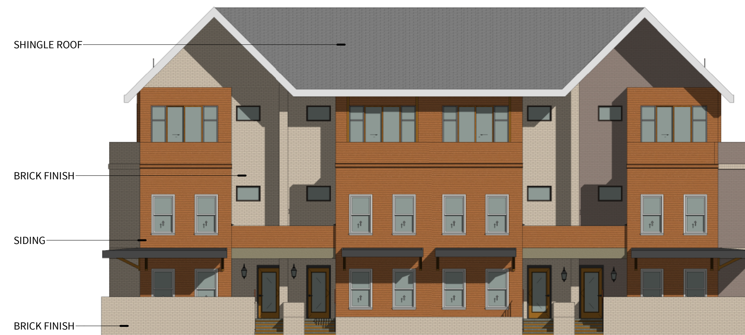
① NORTH ELEVATION - RED BUILDING TYPE SCALE: 1/8" = 1'-0"
