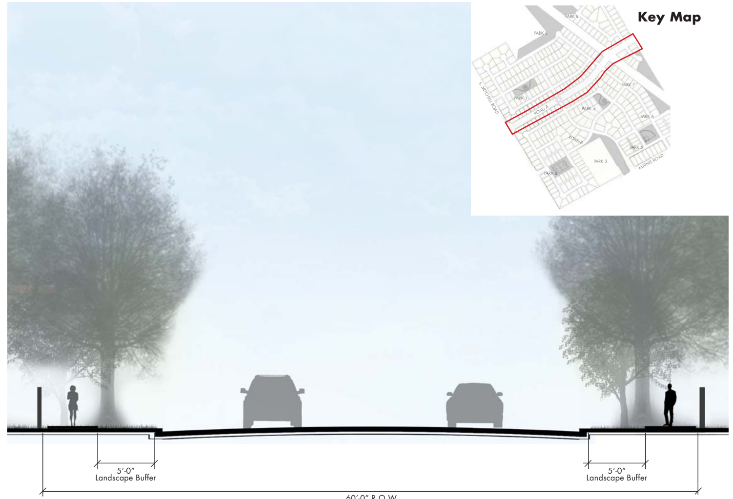
MINOR COLLECTOR ELEVATION - CODE COMPLIANT SCALE 3/16"=1'-0"
