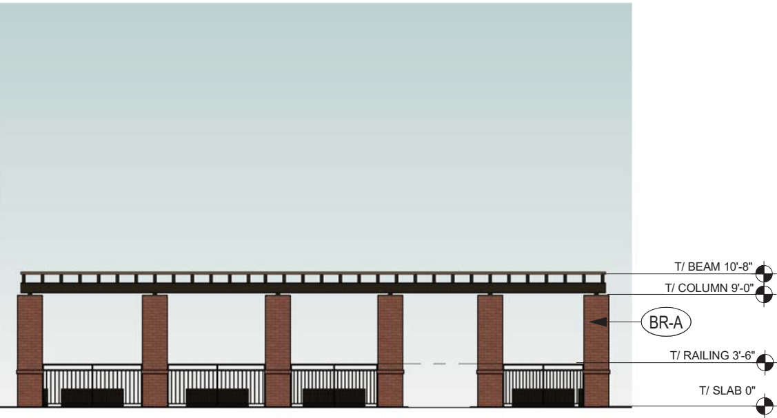
2 TRELLIS - NORTH ELEVATION 3/32" = 1'-0"
