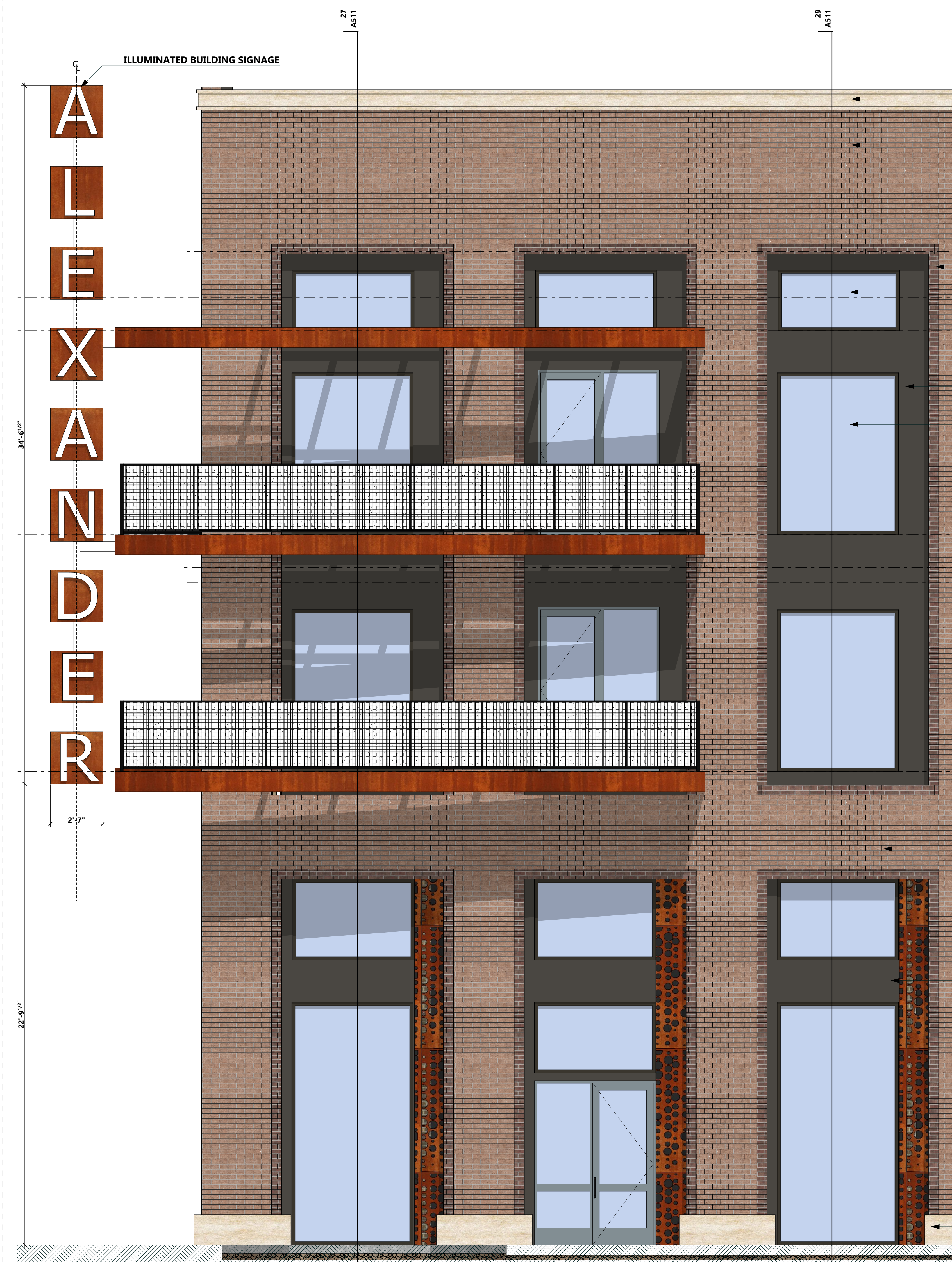
25 | Illuminated Signage Diagram Scale: 3/8" = 1'-0"
