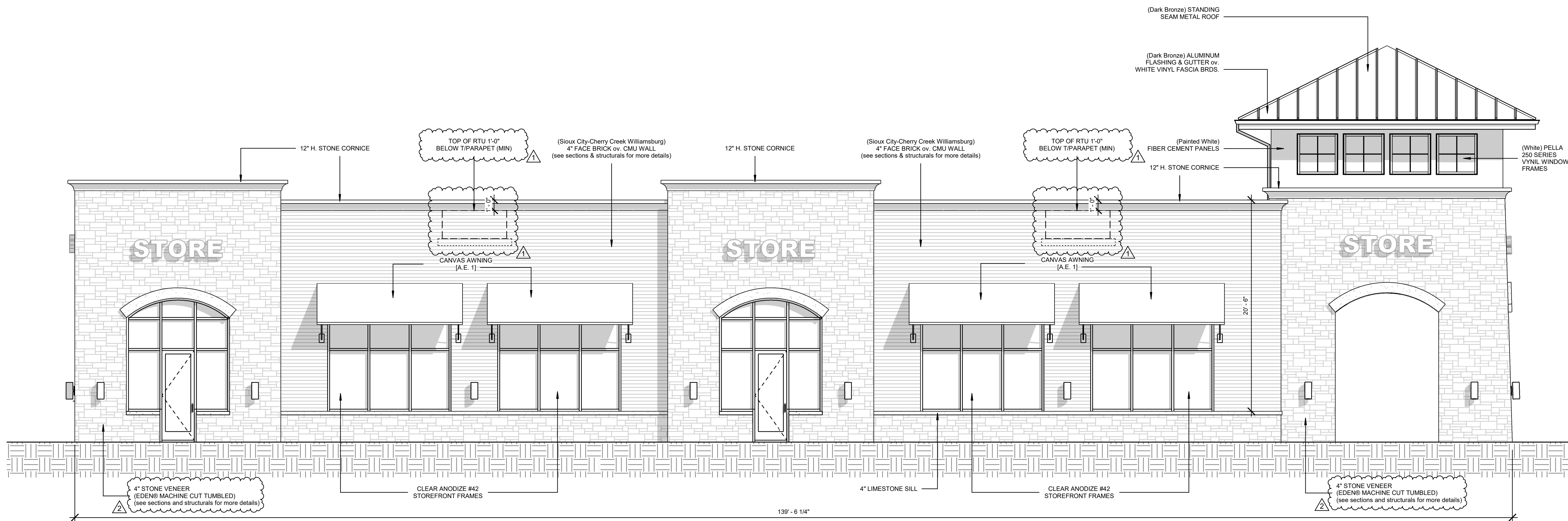
1 East Elevation, Proposed Retail Building #3. SCALE: 3/16" = 1'-0"
