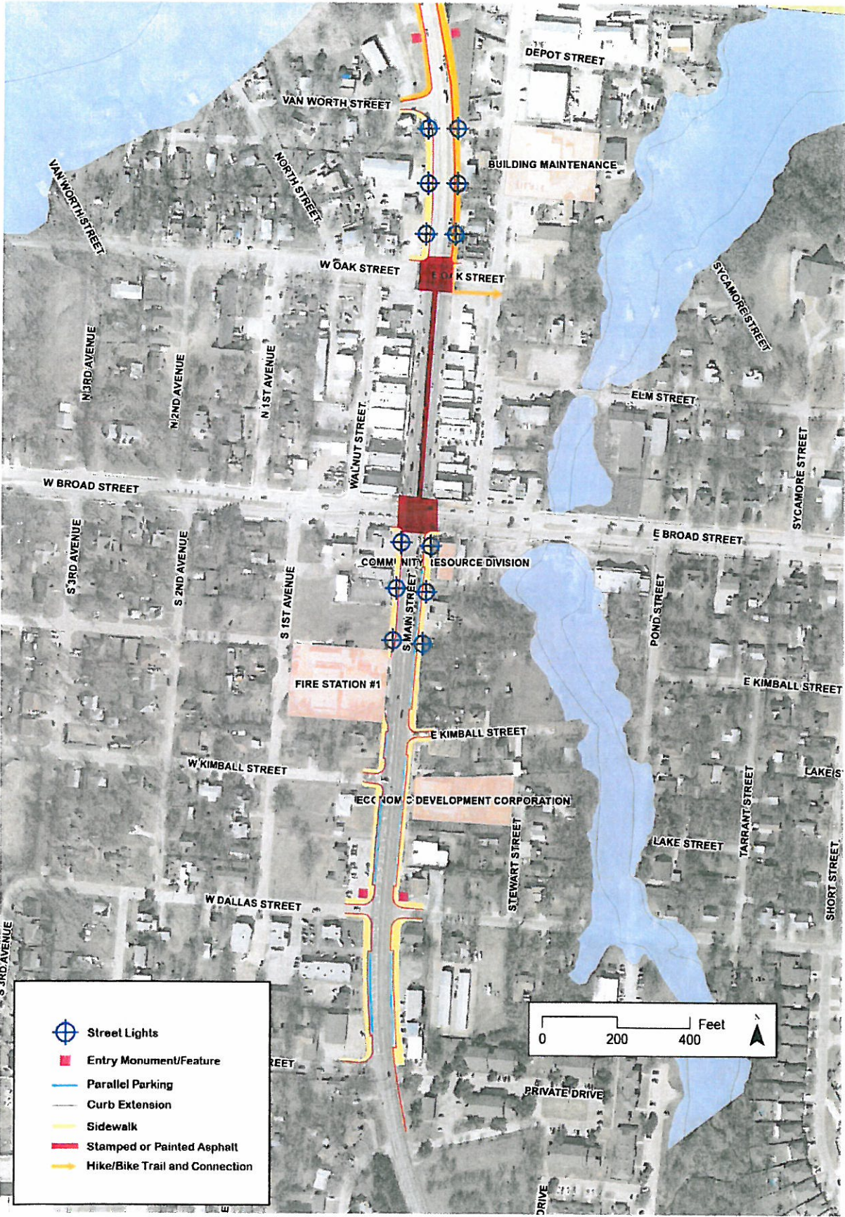
Figure 3b: South Main Street Schematic Improvement Plan
