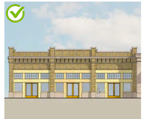
The façade should appear as a flat surface, with any decorative elements and projecting or setback articulations appearing to be subordinate to the dominant form. The decorative pilasters on this building project just enough to define the storefronts but are clearly subordinate to the overall rectangular building form.
