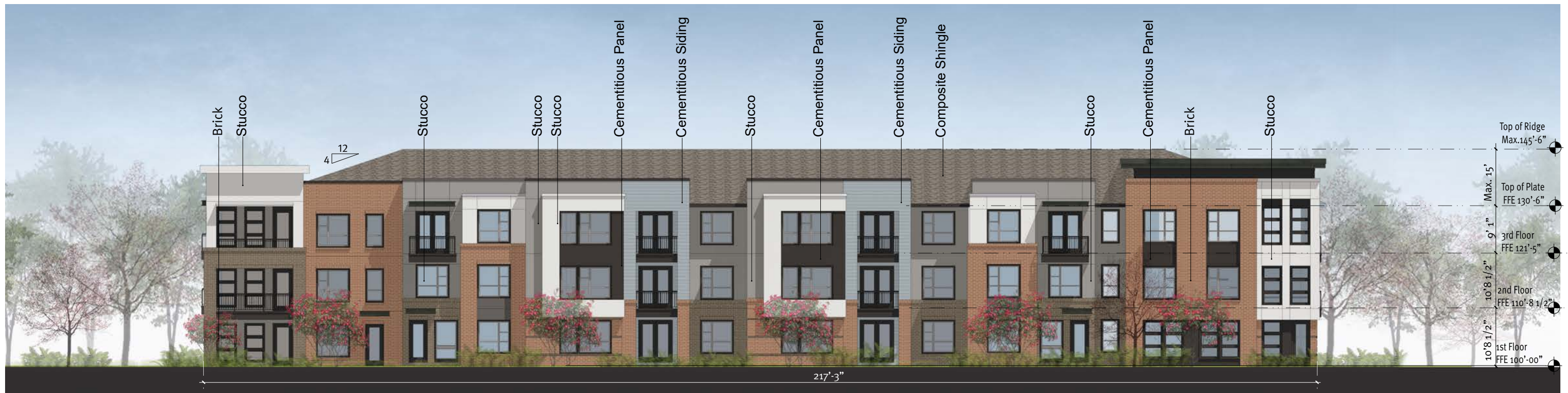
01 Building III - North Elevation
