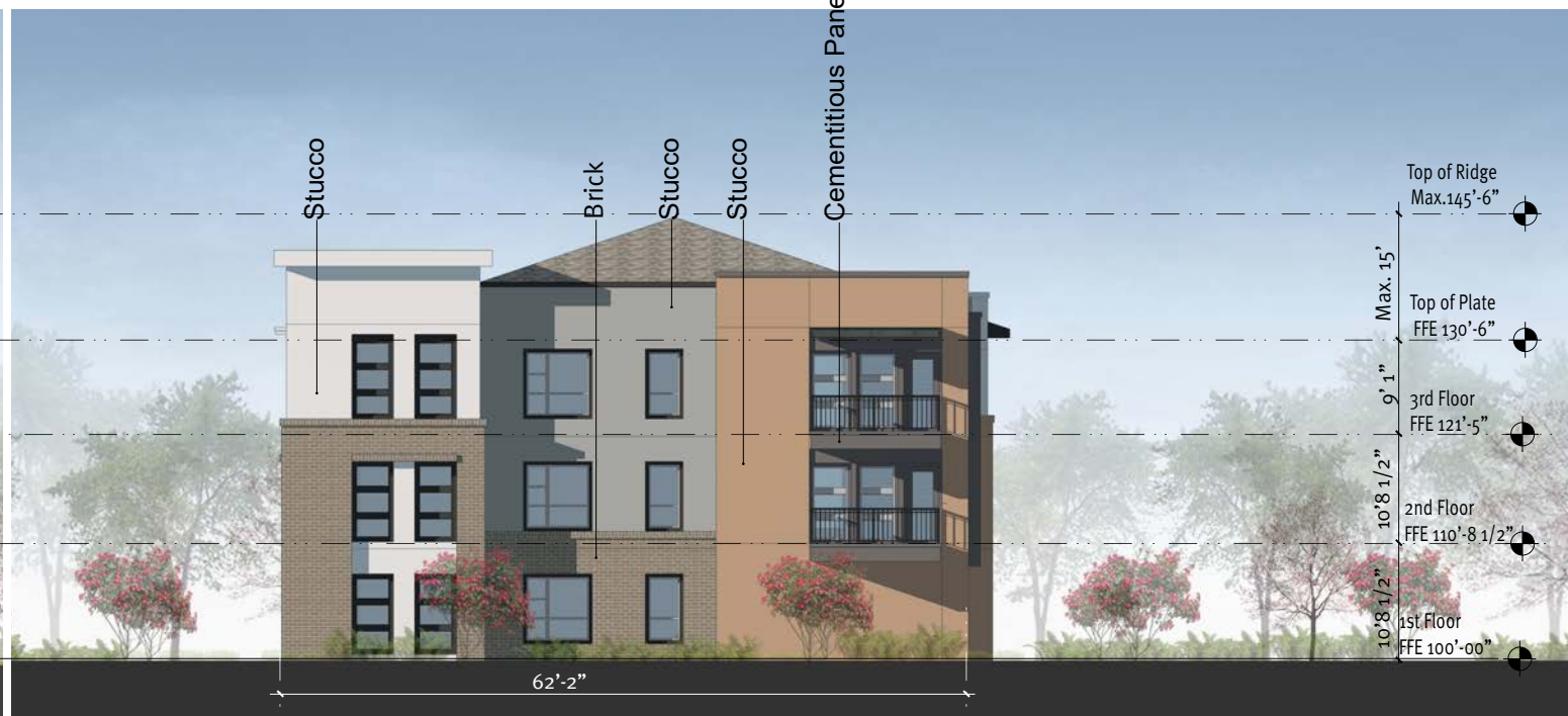
03 Building IV - South Elevation Window 17%
