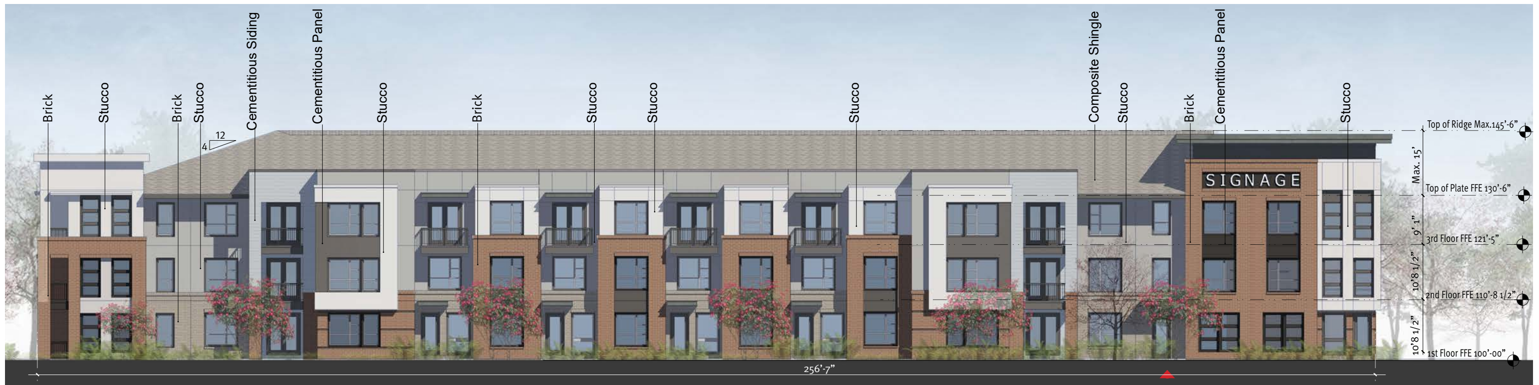
01 Building I - East Elevation
