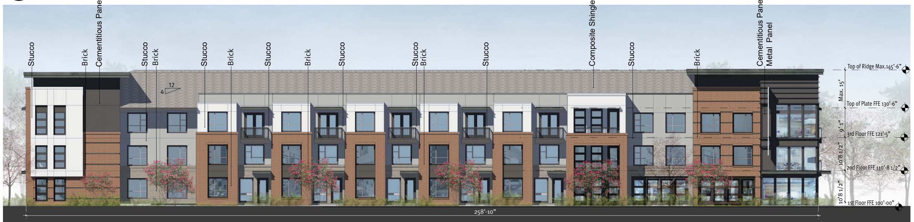
02 Building I - North Elevation
