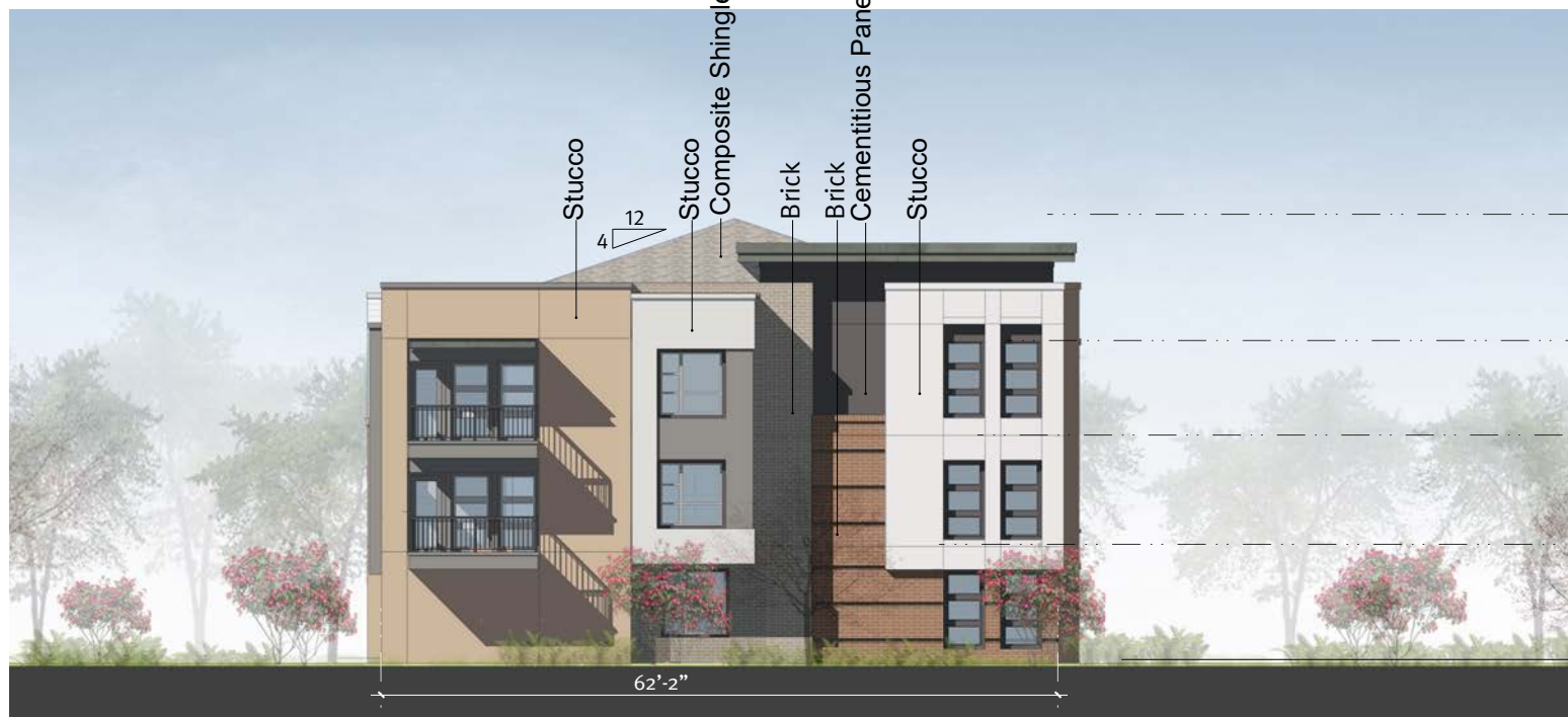
02 Building IV - North Elevation Window 14%
