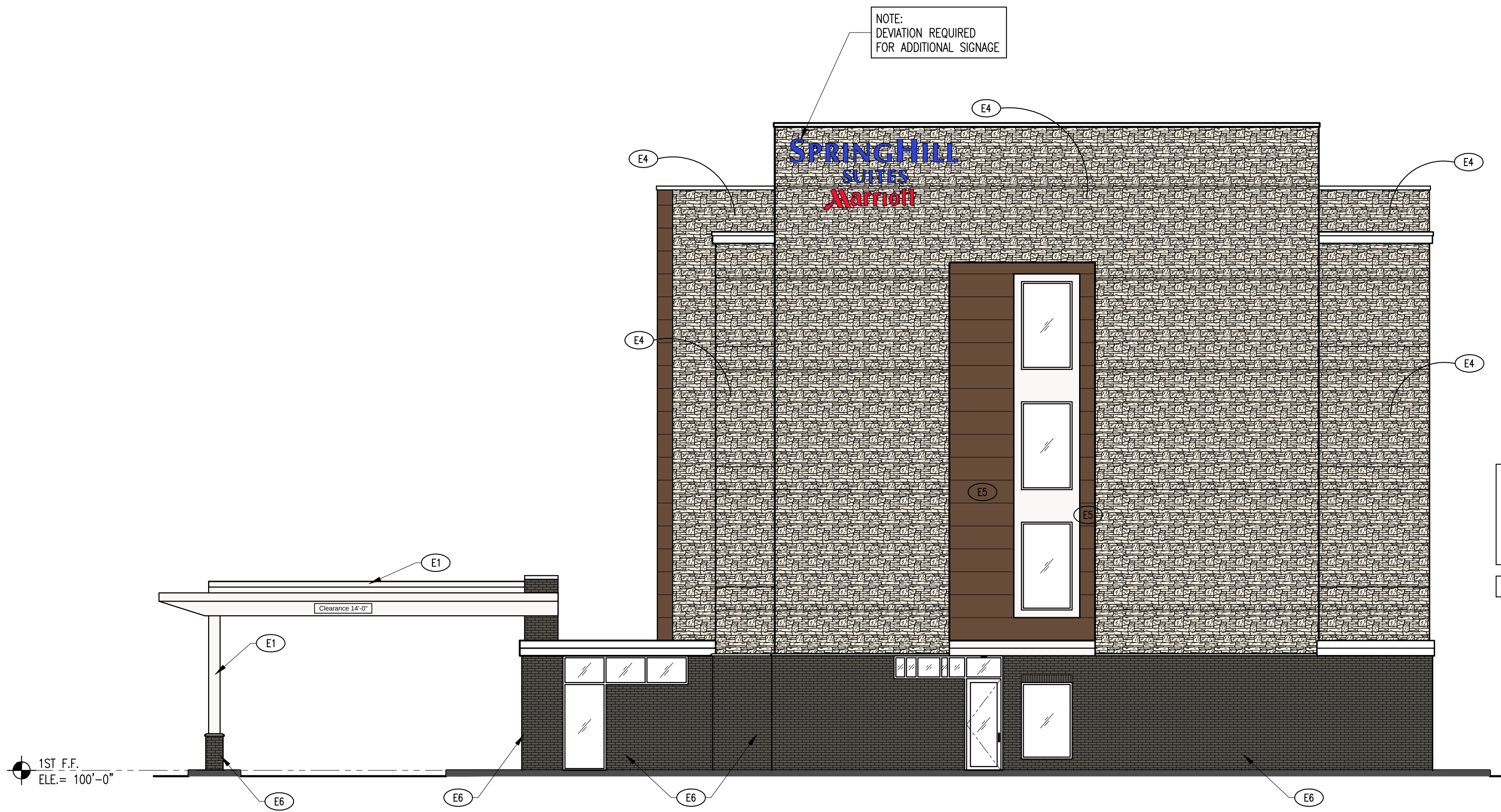
2 BUILDING ELEVATION - NORTH SCALE: 1/8"=1'-0"
