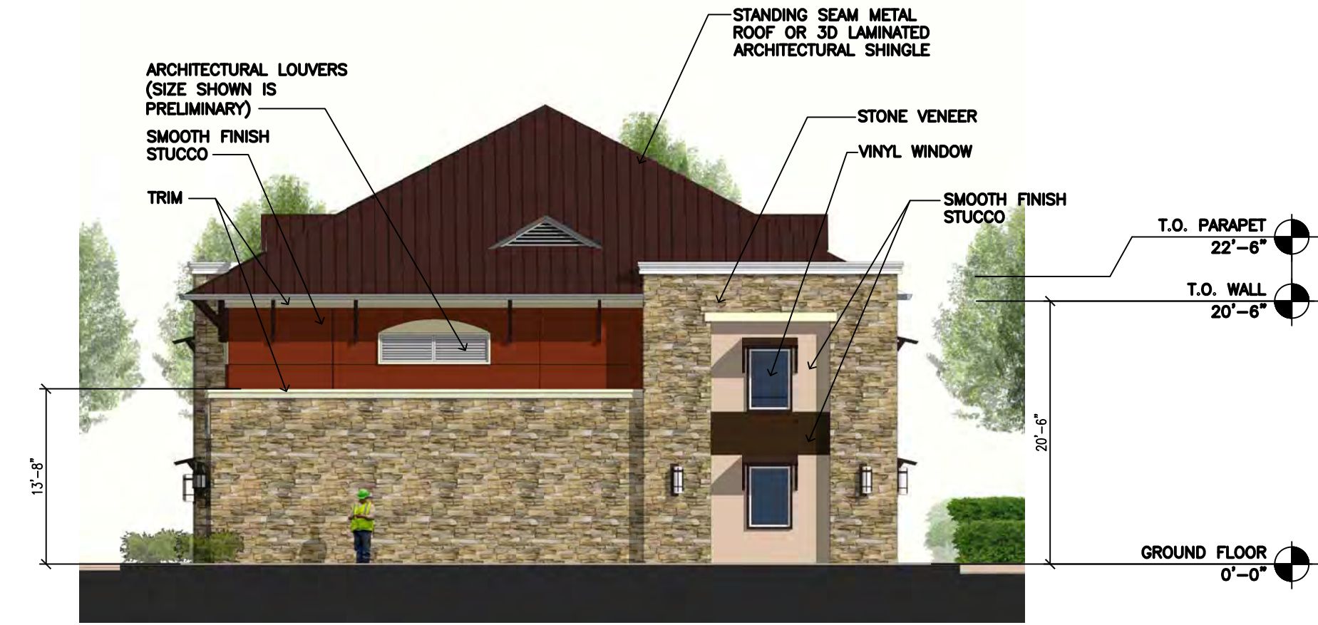
ELEVATION C-C' (NORTH) SCALE 3/32" = 1'-0"
