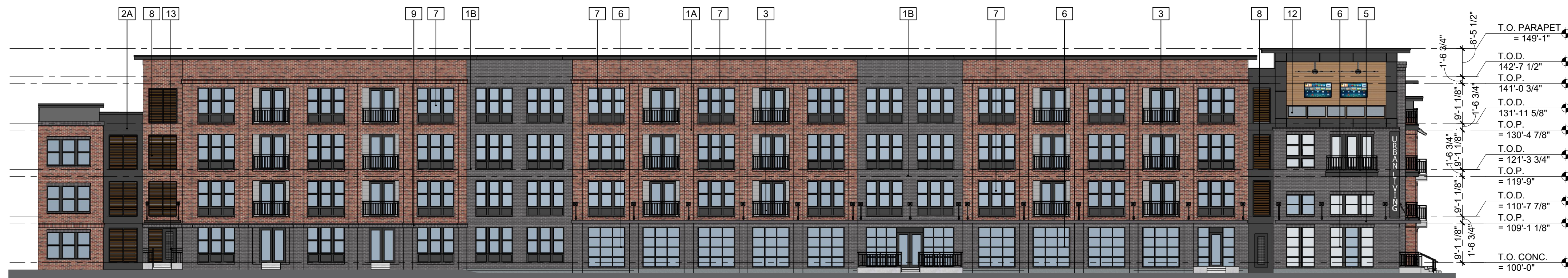
02 BLDG #1 - SOUTHEAST ELEVATION SCALE: 1/16" = 1'-0"
