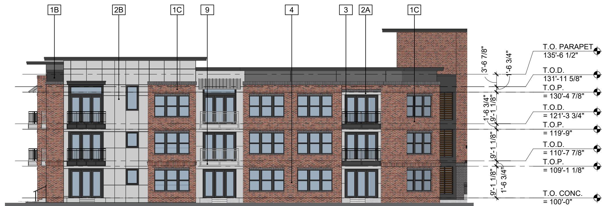
05 BLDG #1 - SOUTH ELEVATION SCALE: 1/16" = 1'-0"
