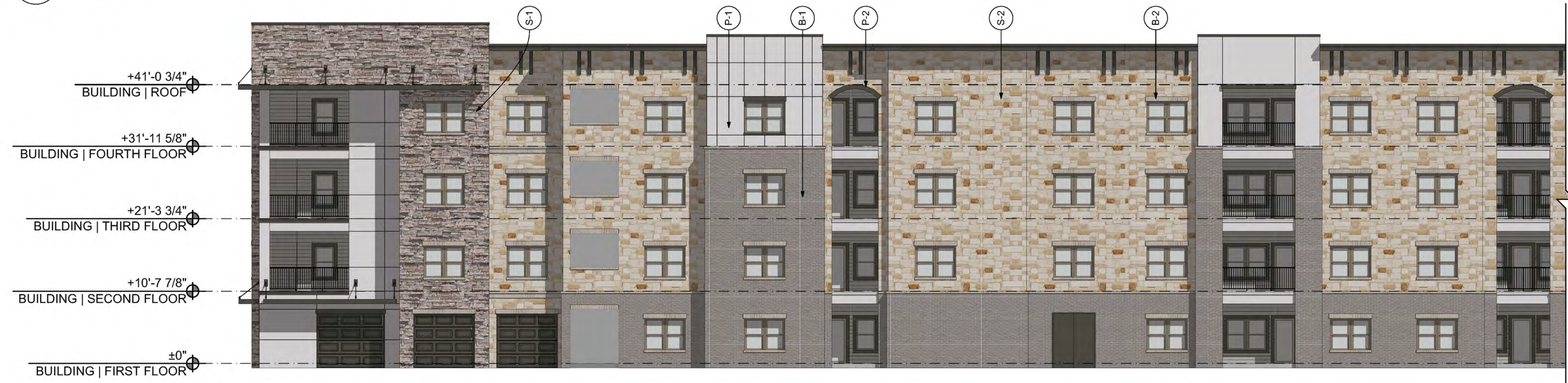
2 BUILDING 2000 - WEST ELEVATION SCALE: 3/32" = 1'-0"
