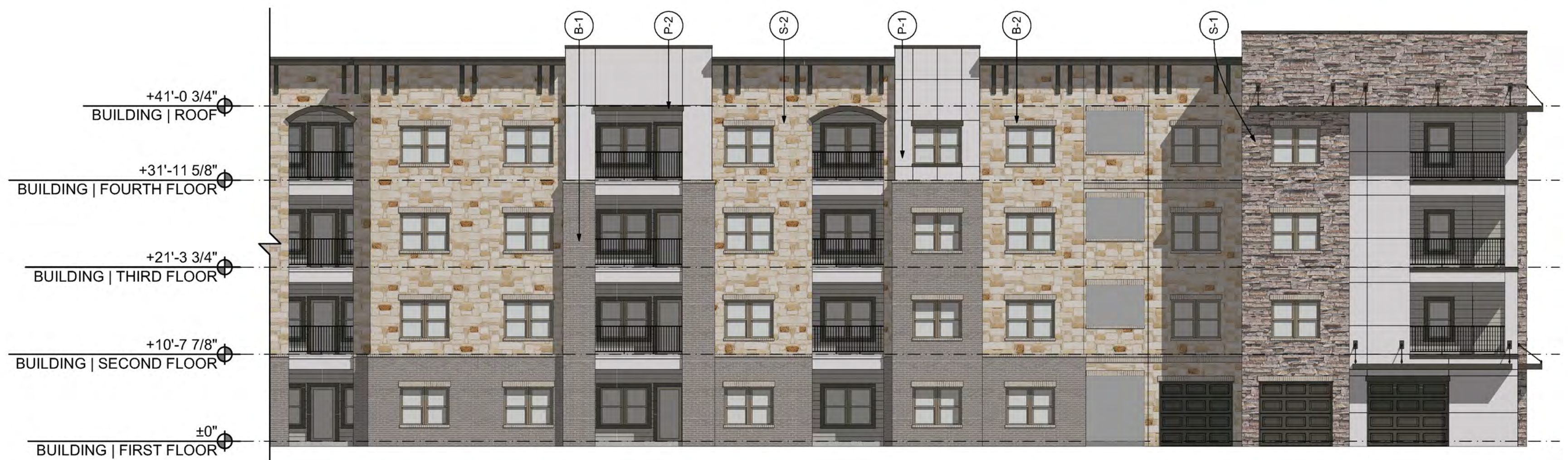
3 BUILDING 2000 - WEST ELEVATION SCALE: 3/32" = 1'-0"
