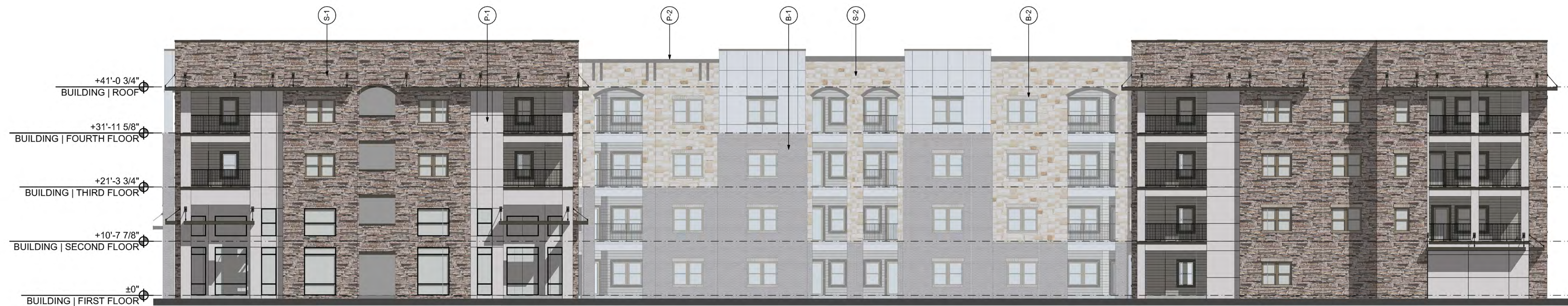
2 BUILDING 1000 - WEST ELEVATION R-2 SCALE: 3/32" = 1'-0"
