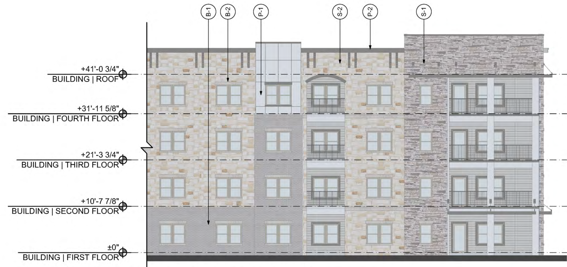
2 BUILDING 3000 - SOUTH ELEVATION SCALE: 3/32" = 1'-0"
