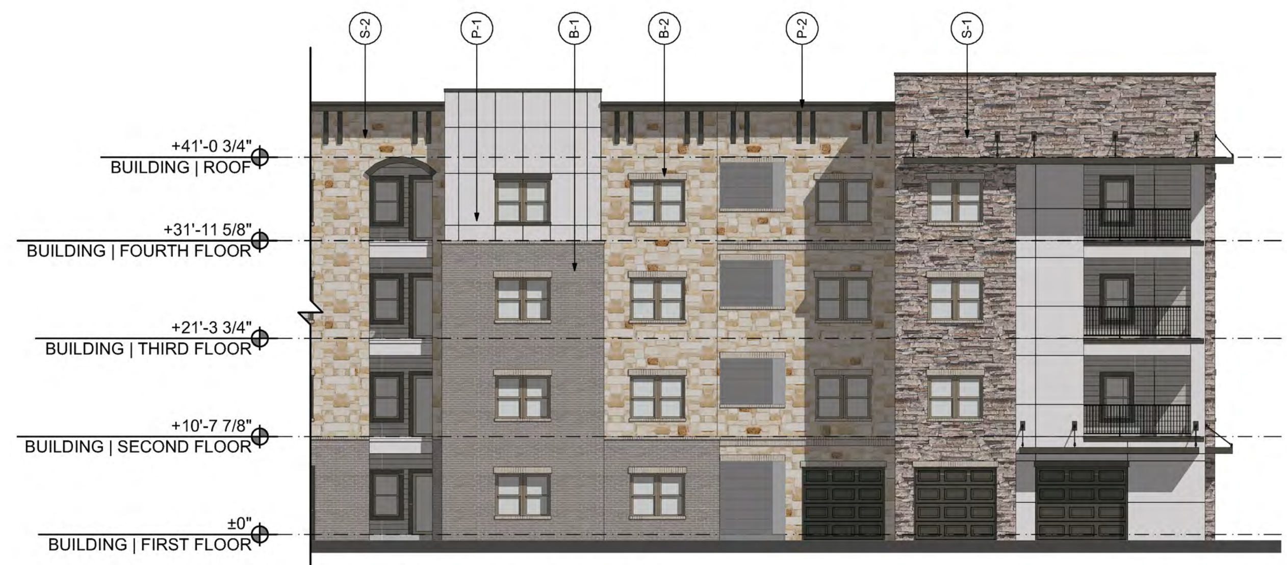
2 BUILDING 3000 - NORTH ELEVATION SCALE: 3/32" = 1'-0"
