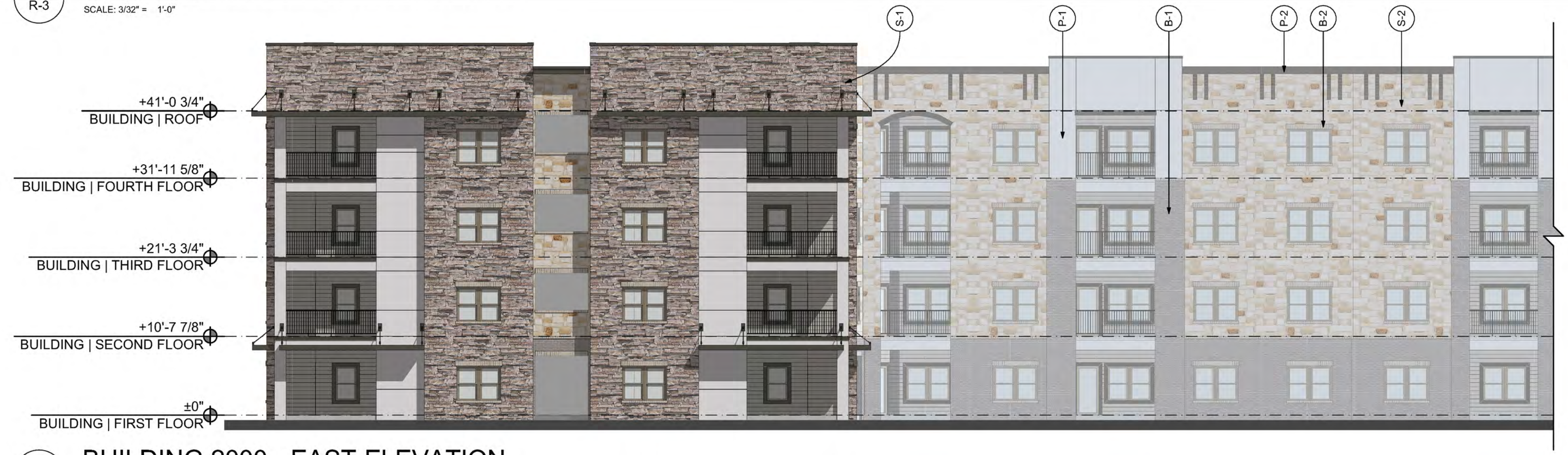
2 BUILDING 2000 - EAST ELEVATION SCALE: 3/32" = 1'-0"
