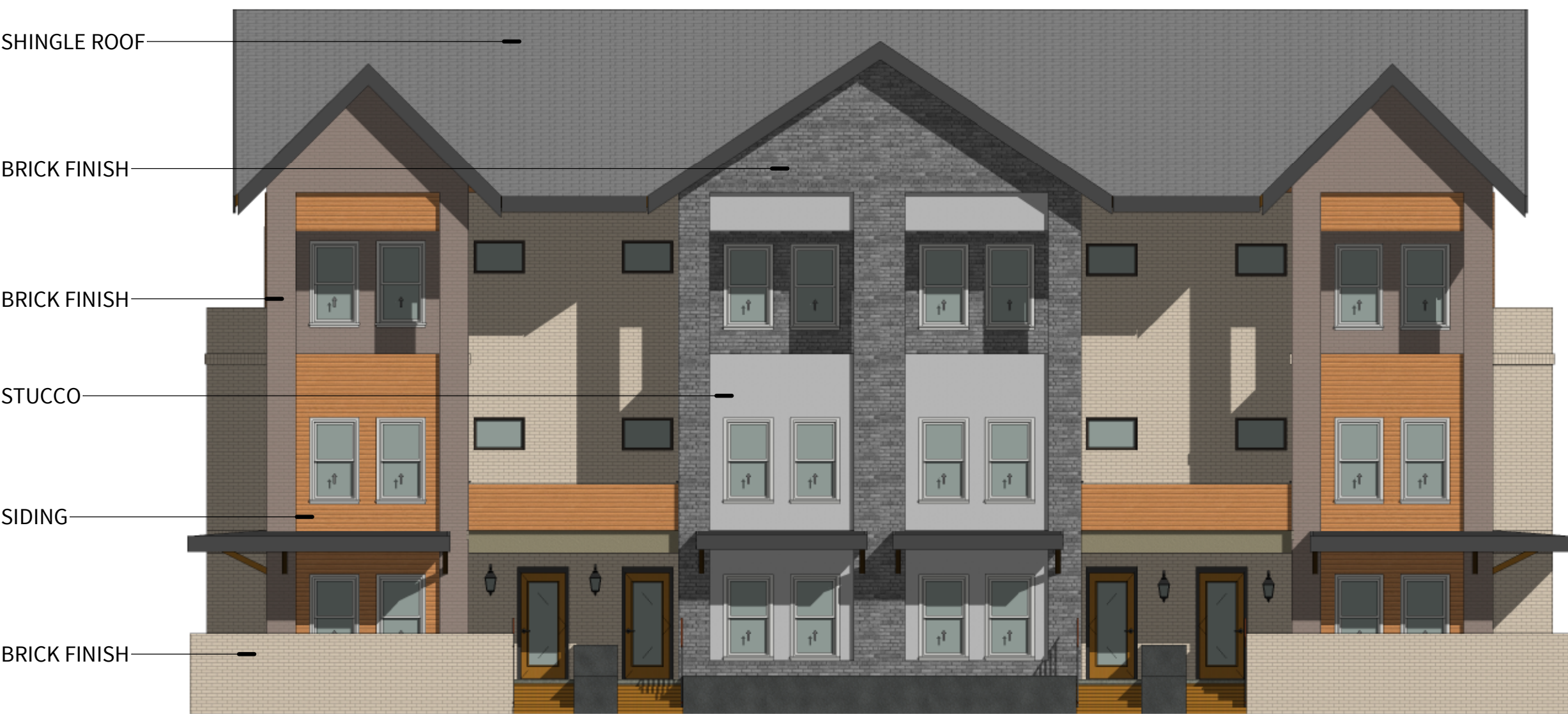
① NORTH ELEVATION - GREEN BUILDING TYPE SCALE: 1/8" = 1'-0"
