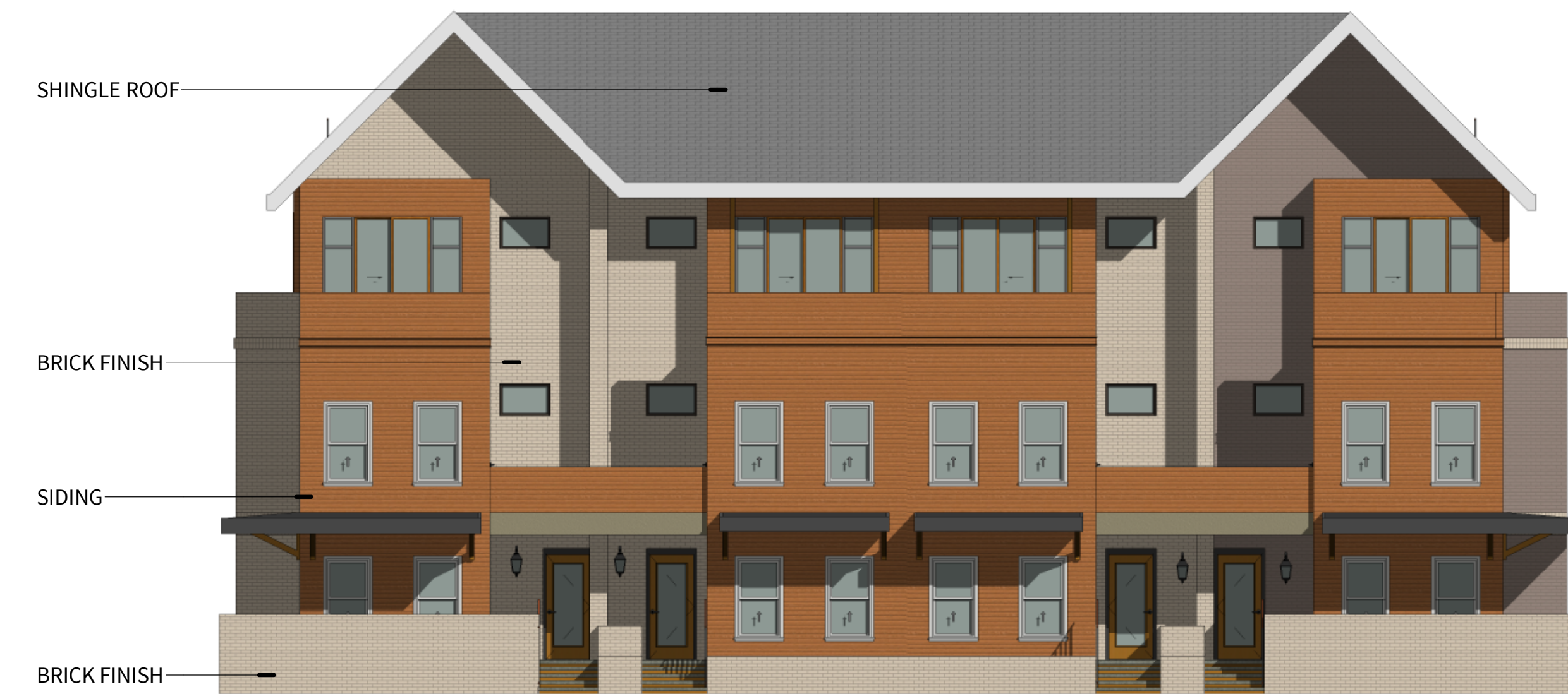
① NORTH ELEVATION - RED BUILDING TYPE SCALE: 1/8" = 1'-0"
