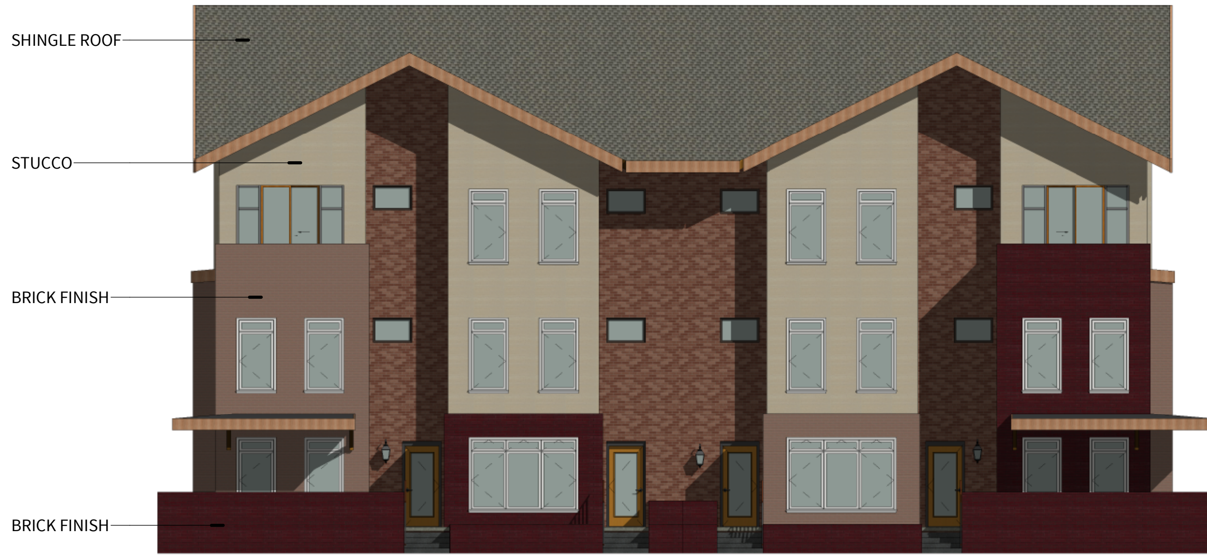
① NORTH ELEVATION - YELLOW BUILDING TYPE SCALE: 1/8" = 1'-0"
