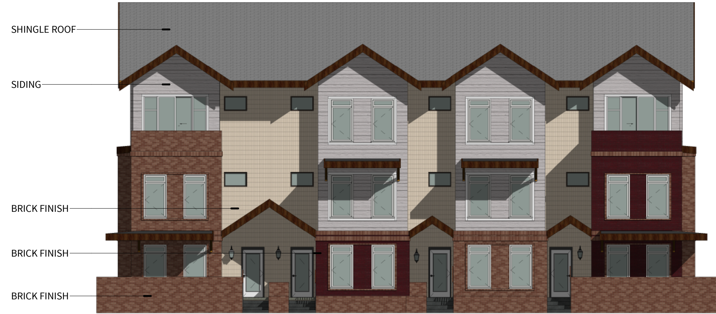
① NORTH ELEVATION - BLUE BUILDING TYPE SCALE: 1/8" = 1'-0"
