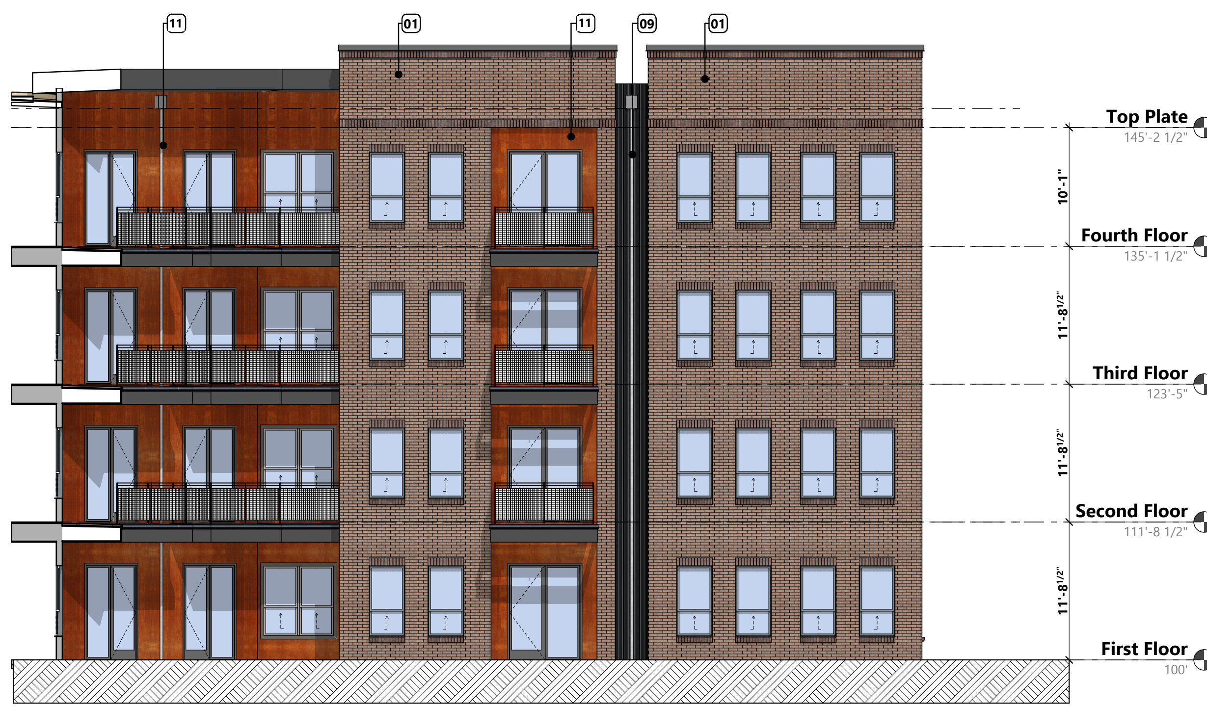
17 | Courtyard 3 East Elevation Scale: 1/8" = 1'-0"
