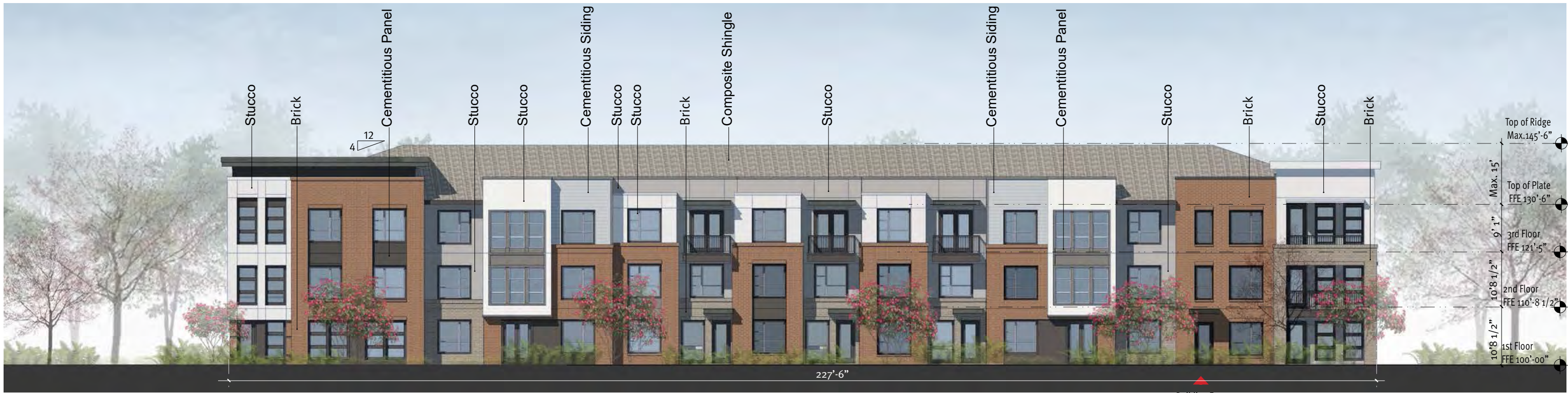
01 Building IV - West Elevation Building Material Percentage: Brick 45% Stucco 29% Cementitious Panel 22% Cementitious Siding 4% Window 27%
