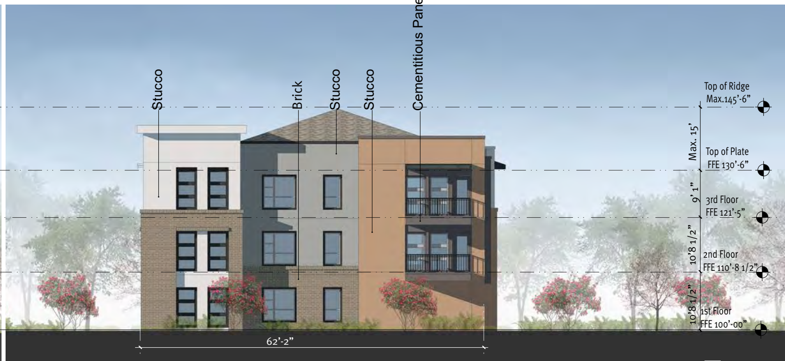
03 Building IV - South Elevation Window 17% Building Material Percentage: Brick 23% Stucco 64% Cementitious Panel 13%
