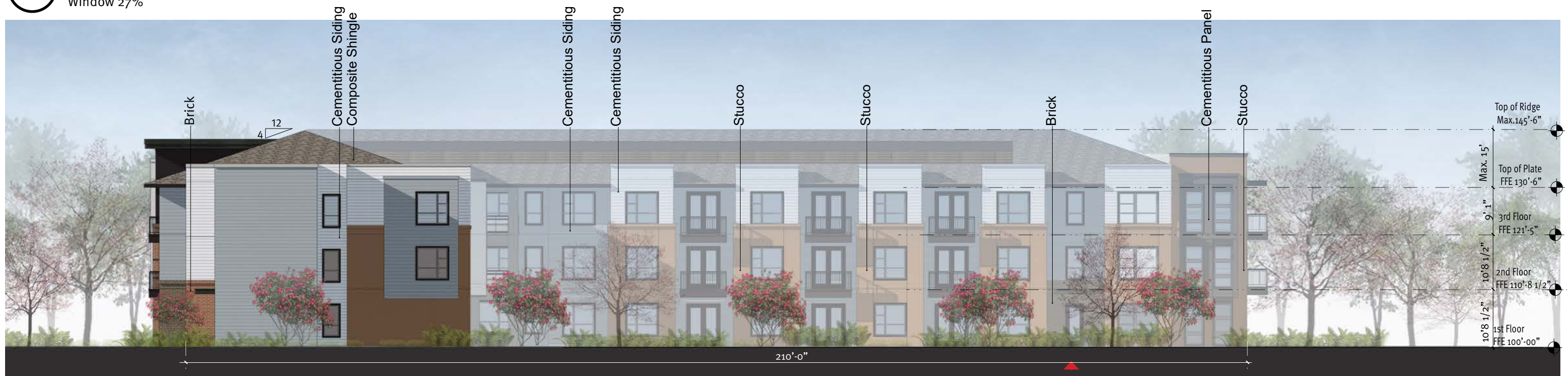
02 Building III - South Elevation Building Material Percentage: Brick 11% Stucco 35% Cementitious Panel 11% Cementitious Siding 43% Window 16%
