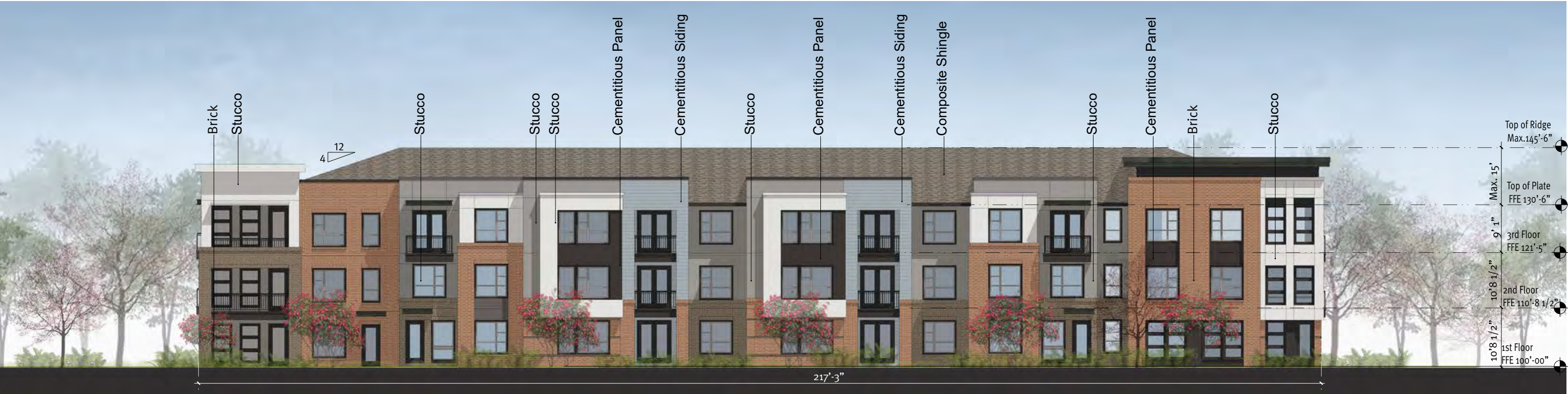
01 Building III - North Elevation Building Material Percentage: Brick 40% Stucco 31% Cementitious Panel 22% Cementitious Siding 7% Window 24%
