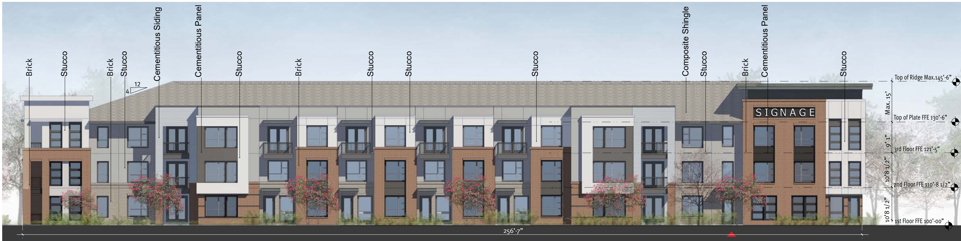
01 Building I - East Elevation Window 25% Building Material Percentage: Brick 44% Stucco 25% Cementitious Panel 24% Cementitious Siding 7%
