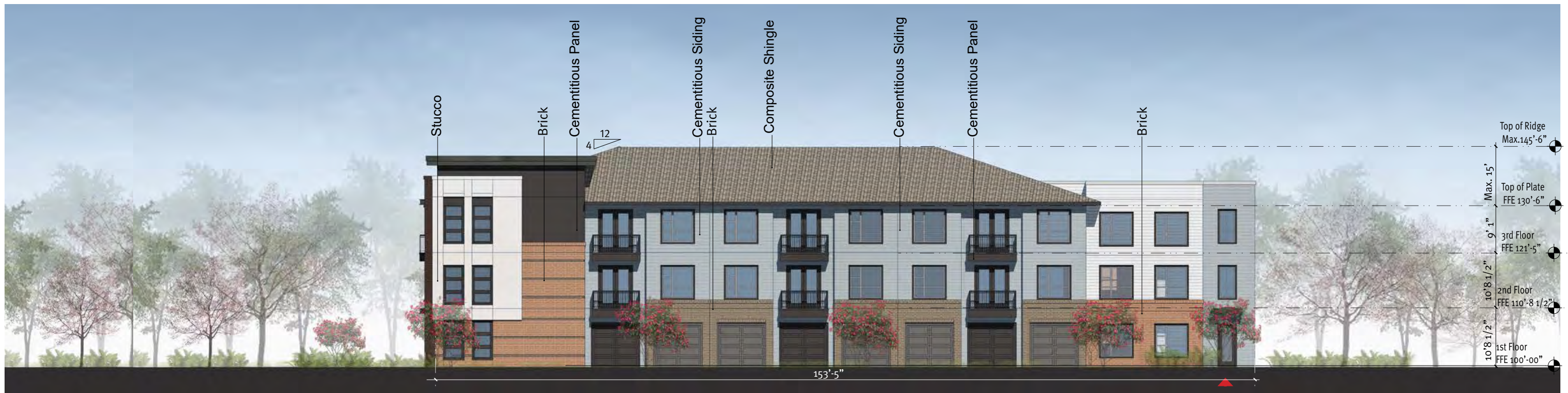
01 Building III - West Elevation Building Material Percentage: Brick 23% Stucco 18% Cementitious Panel 19% Cementitious Siding 40% Window 27%
