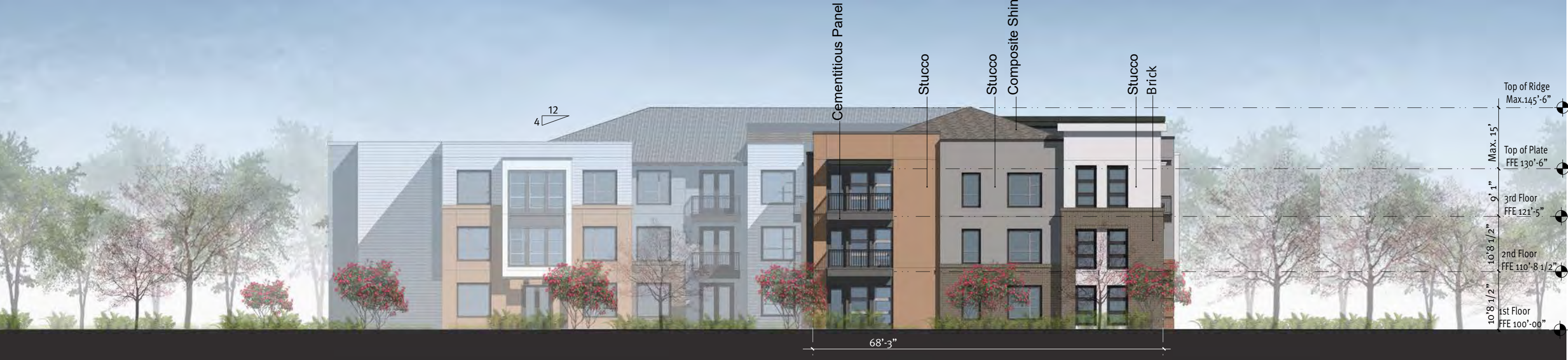
02 Building III - East Elevation Building Material Percentage: Brick 15% Stucco 47% Cementitious Panel 20% Cementitious Siding 18% Window 22%
