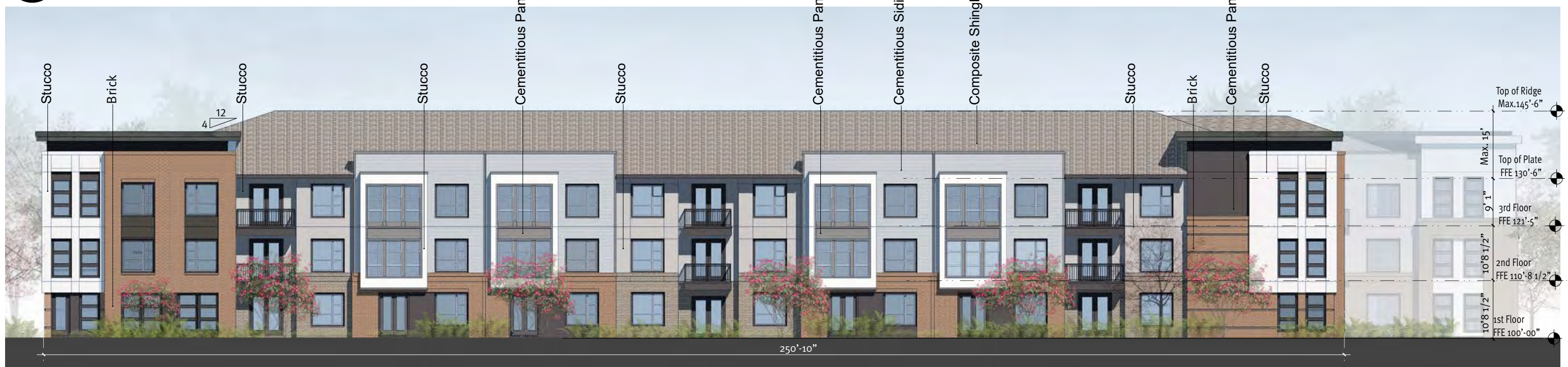
02 Building II - East Elevation Building Material Percentage: Brick 30% Stucco 26% Cementitious Panel 29% Cementitious Siding 15% Window 24%
