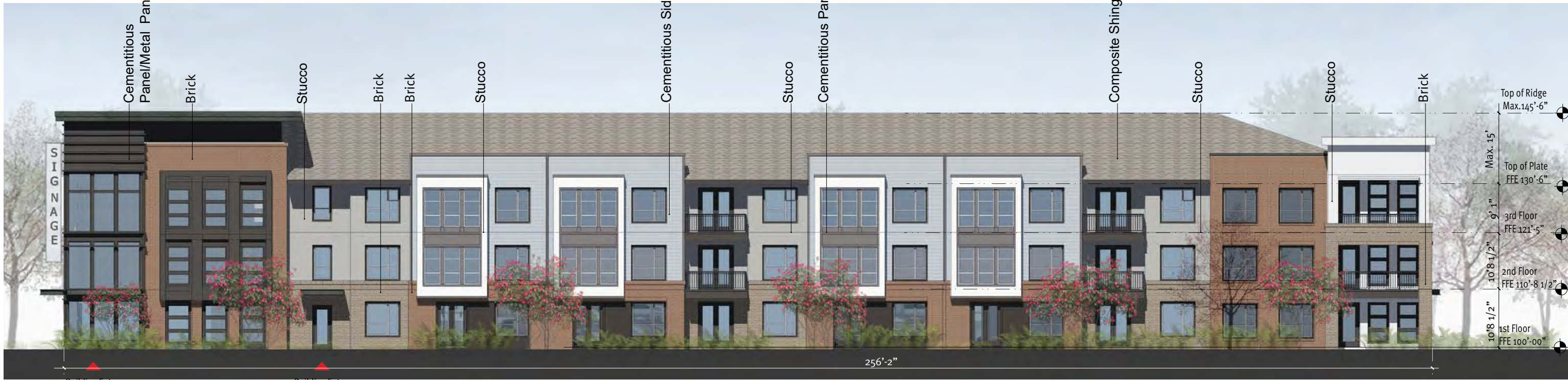
02 Building I - West Elevation Window 27% Building Material Percentage: Brick 31% Stucco 21% Cementitious Panel 33% Cementitious Siding 15%
