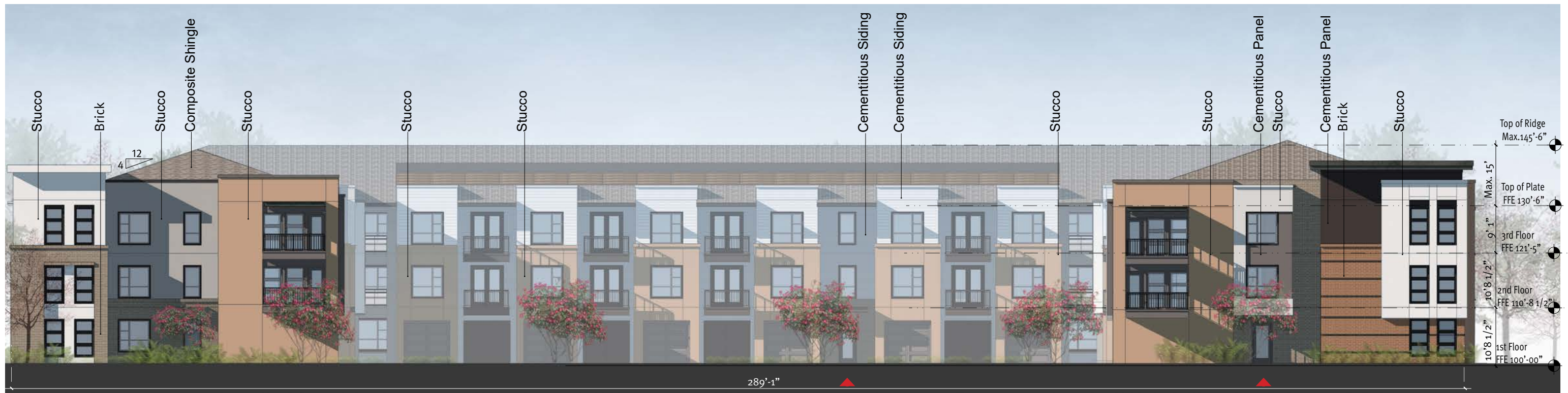
01 Building II - South Elevation Building Material Percentage: Brick 14% Stucco 47% Cementitious Panel 18% Cementitious Siding 21% Window 22%
