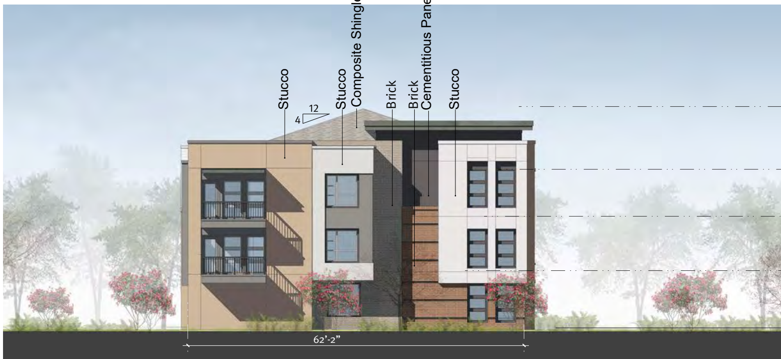
02 Building IV - North Elevation Window 14% Building Material Percentage: Brick 25% Stucco 51% Cementitious Panel 24%
