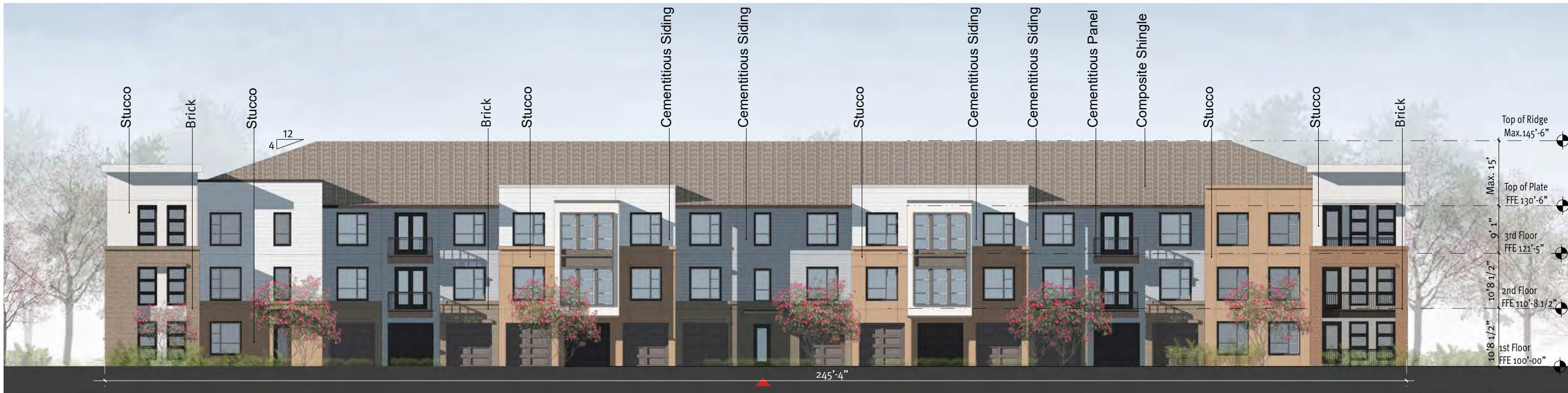
01 Building I - South Elevation Window 38% Building Material Percentage: Brick 18% Stucco 13% Cementitious Panel 19% Cementitious Siding 50%
