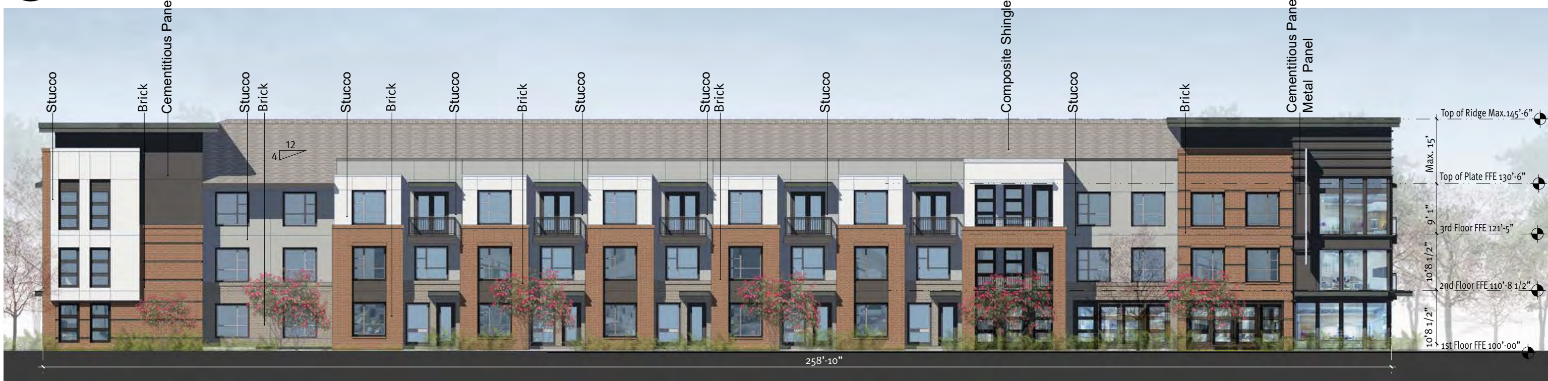
02 Building I - North Elevation Window 24% Building Material Percentage: Brick 38% Stucco 32% Cementitious Panel 30%
