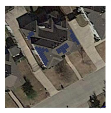
If we are not allowed to utilize the front of our home for solar panels, we will be able to install 20 solar panels on the sides of the home. With 20 panels we will only be able to produce **6588 kWh** of electricity per year. (Image below).
