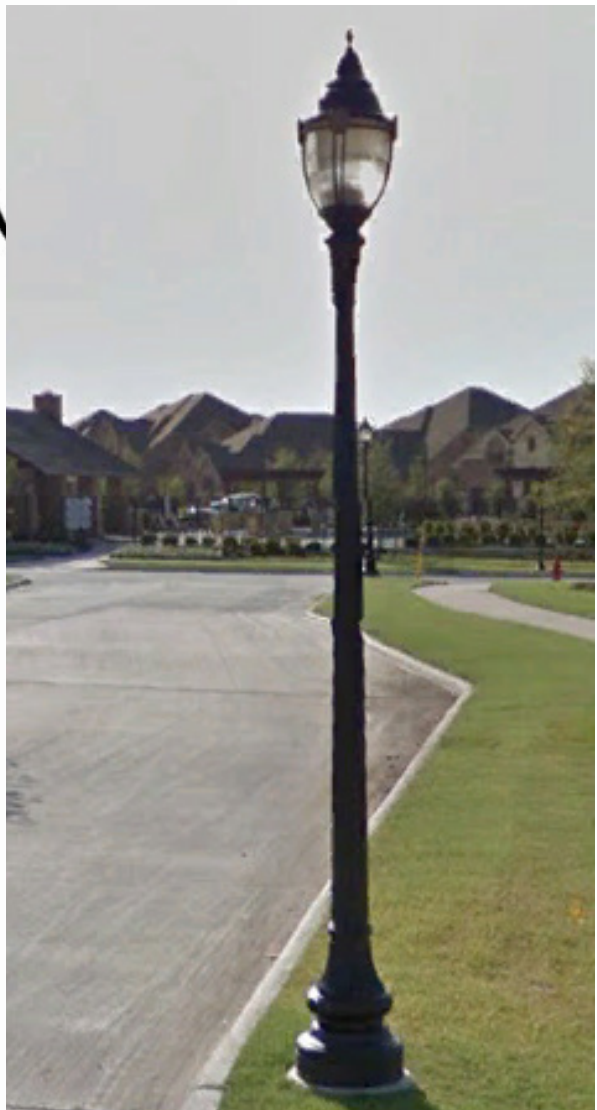
11' TALL ONCOR LIGHT STANDARD - AMERICAN POLE WITH FRISCO LUMINAIRE* (NOTE* THE ACORN LUMINAIRE MAYBE USED AS AN ALTERNATIVE TO THE FRISCO LUMINAIRE.)
