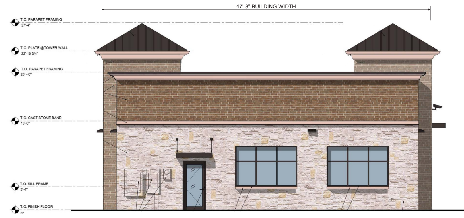
Side (Left) Elevation - 1/8"=1'-0"
