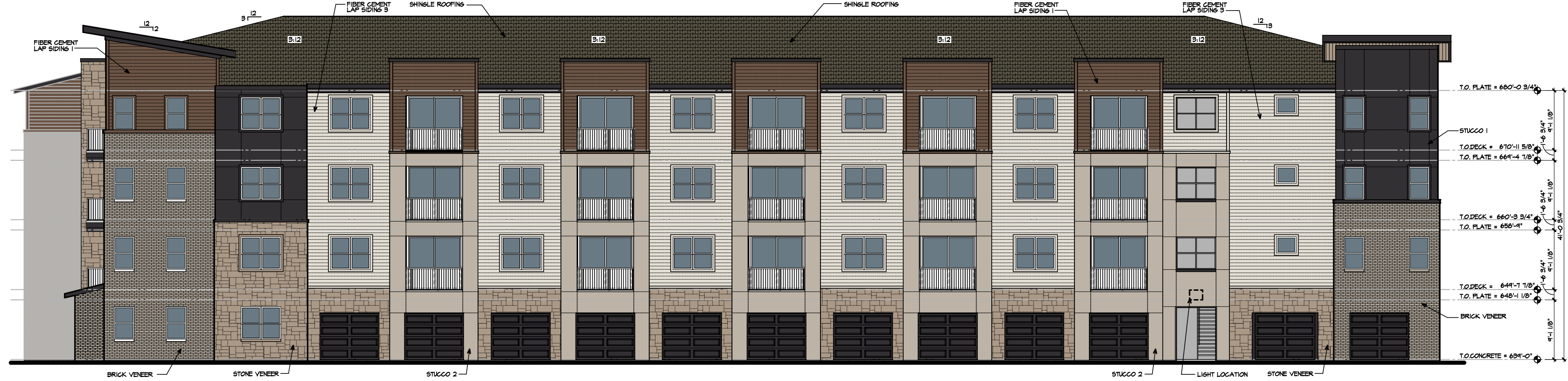
03 EAST ELEVATION BUILDING 300 SCALE: 3/32"=1'-0"
