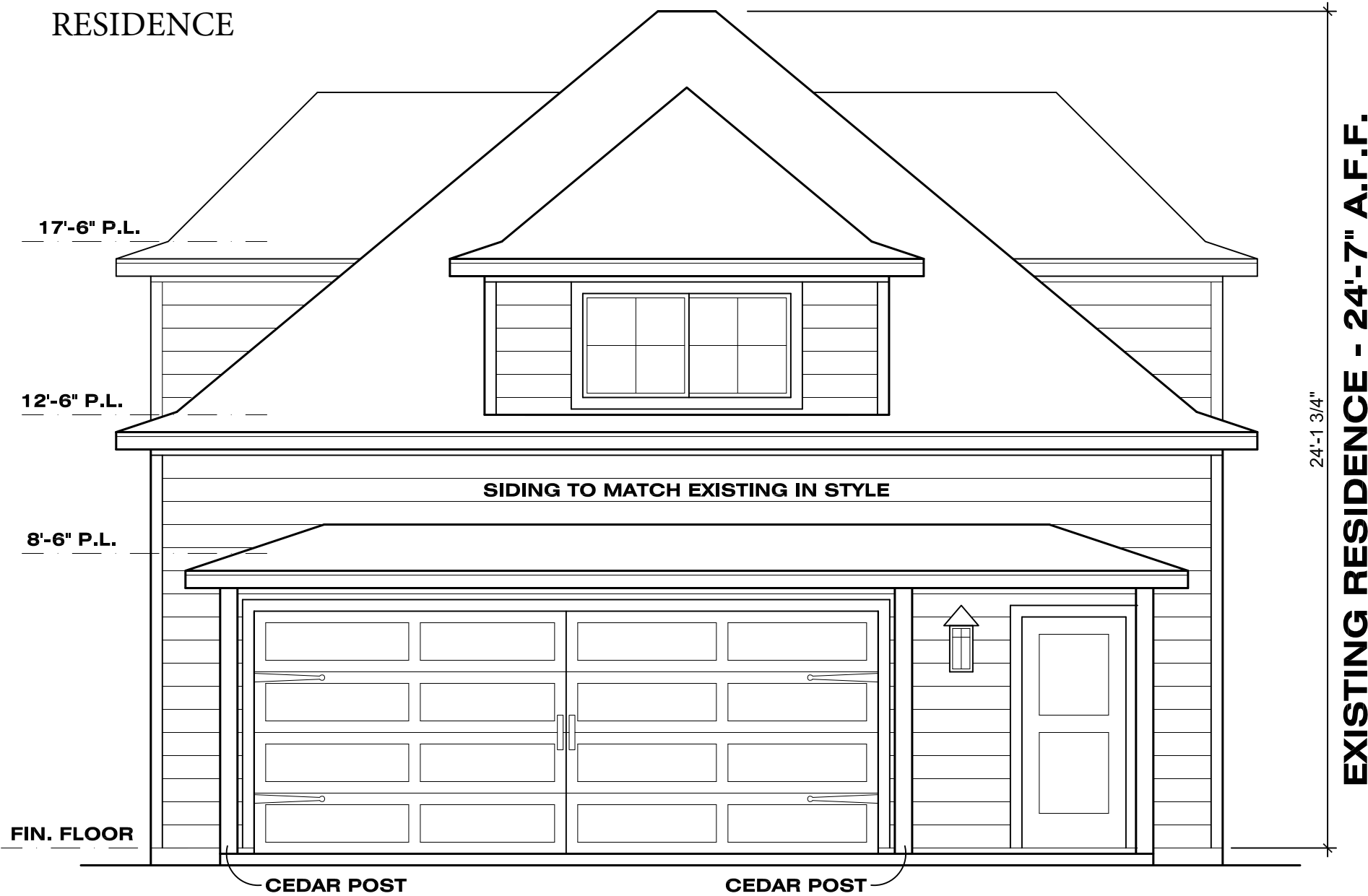
FRONT ELEVATION SCALE:1/4"=1'-0" CEMENTITIOUS SIDING AND TRIM, TYP.
