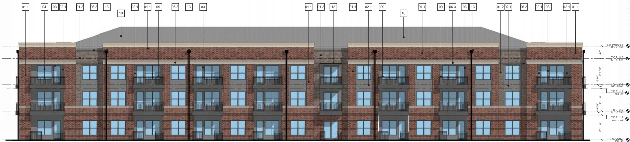
01 NORTH ELEVATION SCALE: 3/32" = 1'-0"
