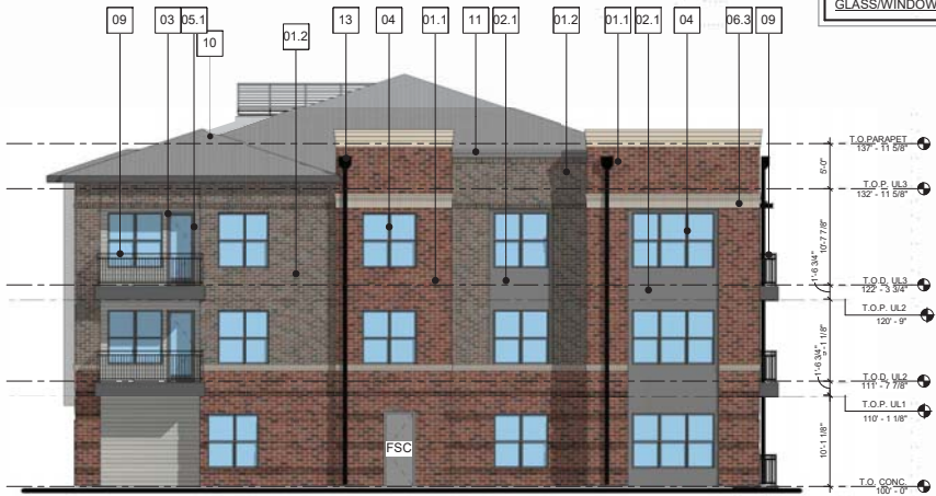
02 NORTH ELEVATION SCALE: 3/32" = 1'-0"
