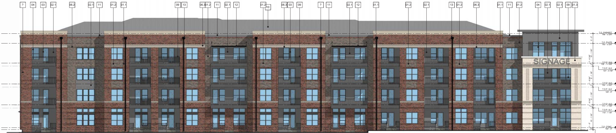
01 EAST ELEVATION SCALE: 3/32" = 1'-0"
