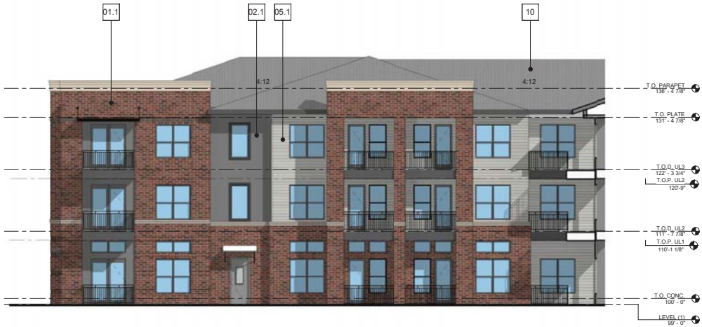
02 EAST ELEVATION 01 SCALE: 3/32" = 1'-0"
