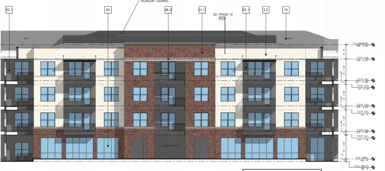
02 SOUTH ELEVATION 02 SCALE: 3/32" = 1'-0"
