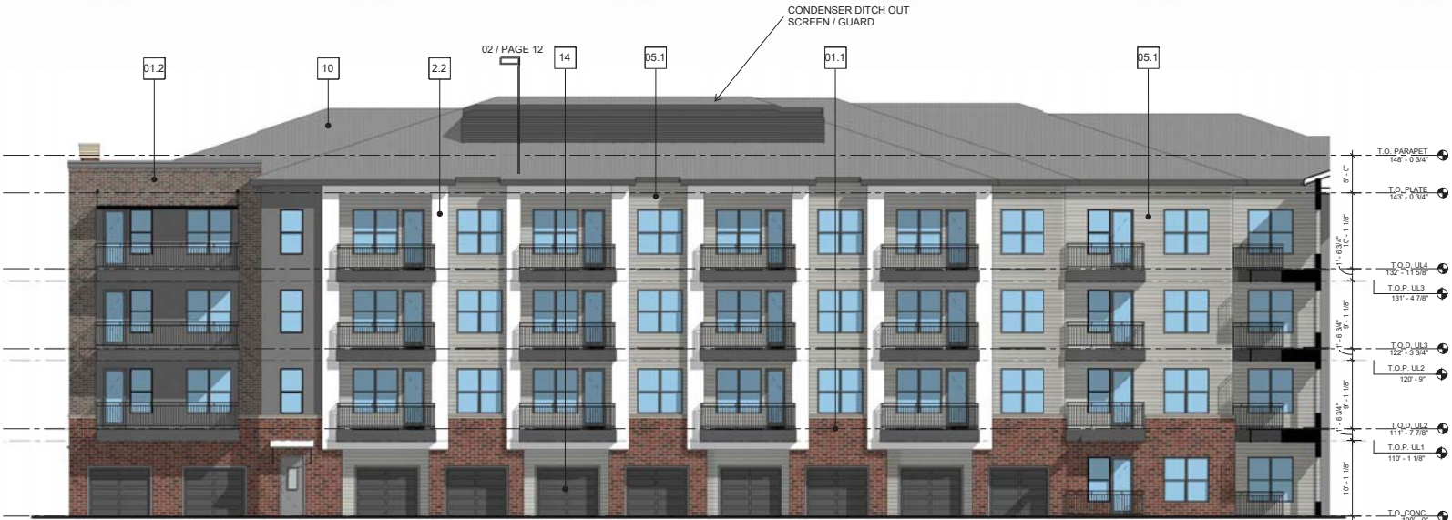
2 SOUTH ELEVATION-1 SCALE: 3/32" = 1'-0"
