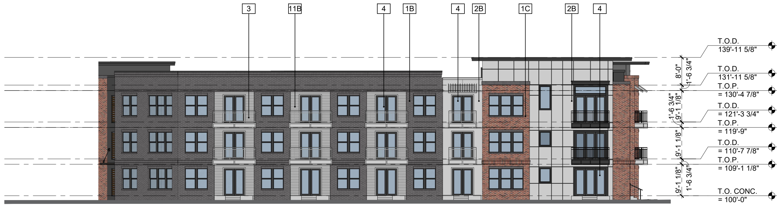
04 BLDG #1 - NORTH ELEVATION SCALE: 1/16" = 1'-0"
