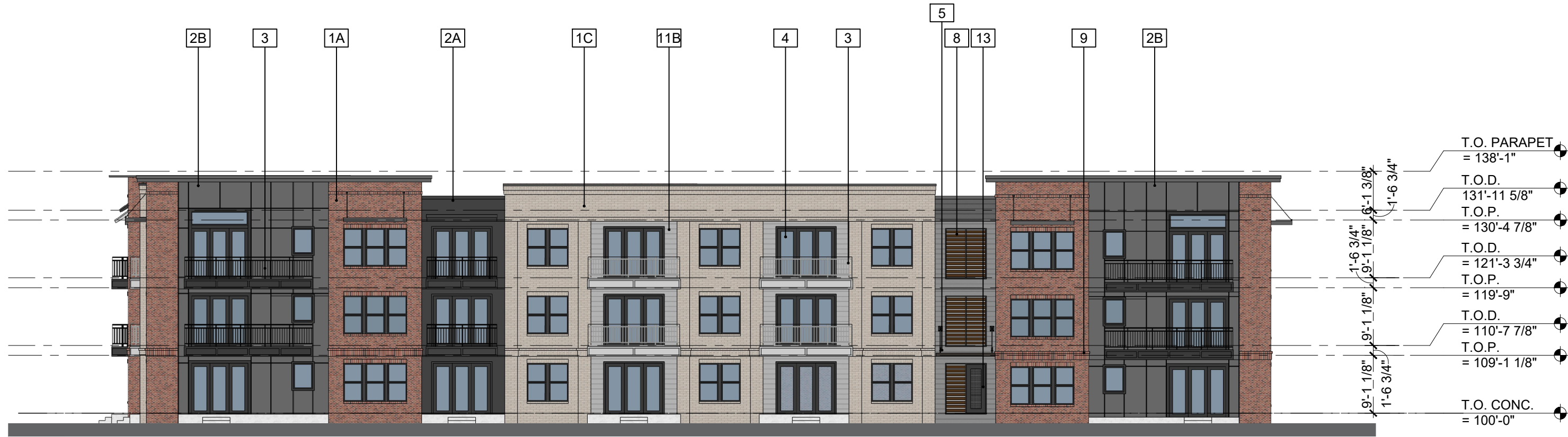
04 BLDG #2 & 3- WEST ELEVATION SCALE: 1/16" = 1'-0"
