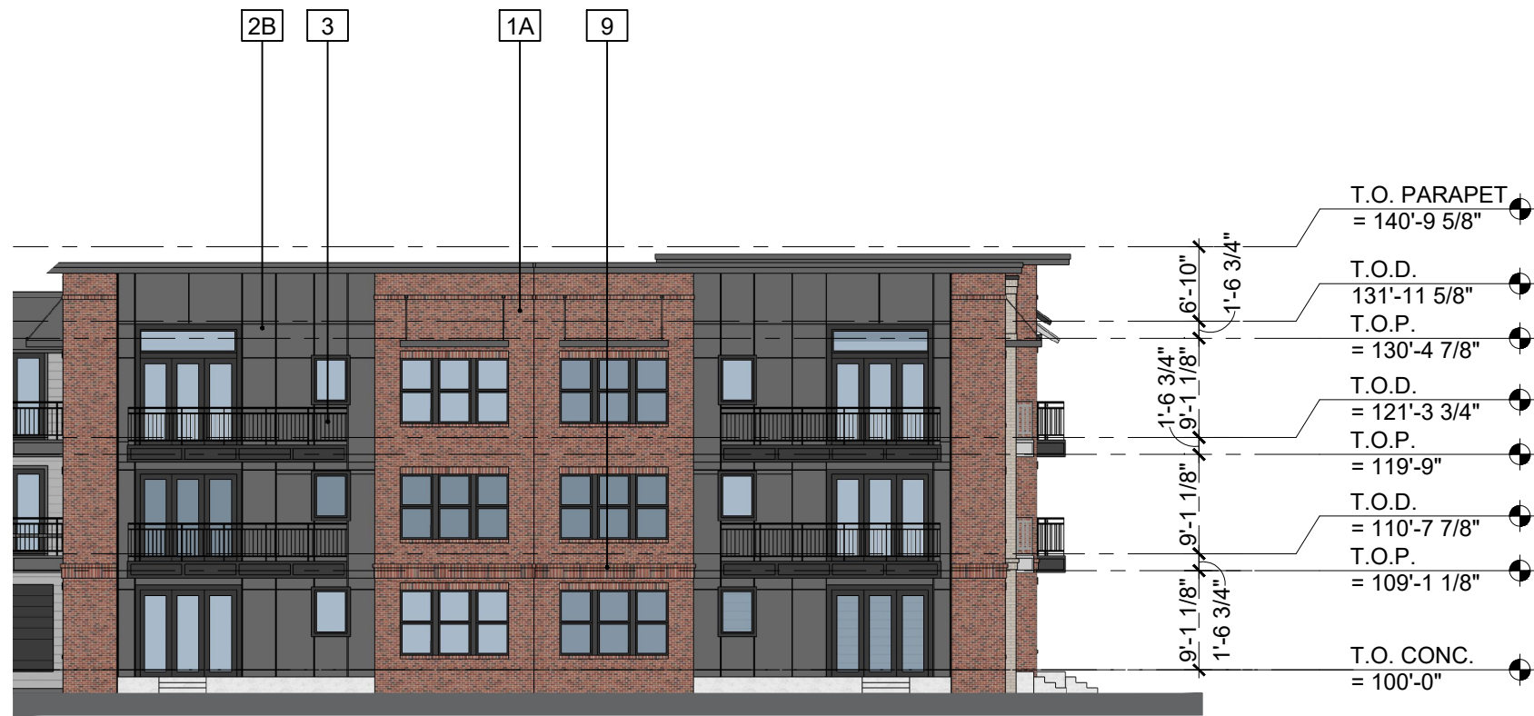
05 BLDG #2 & 3 - EAST ELEVATION SCALE: 1/16" = 1'-0"
