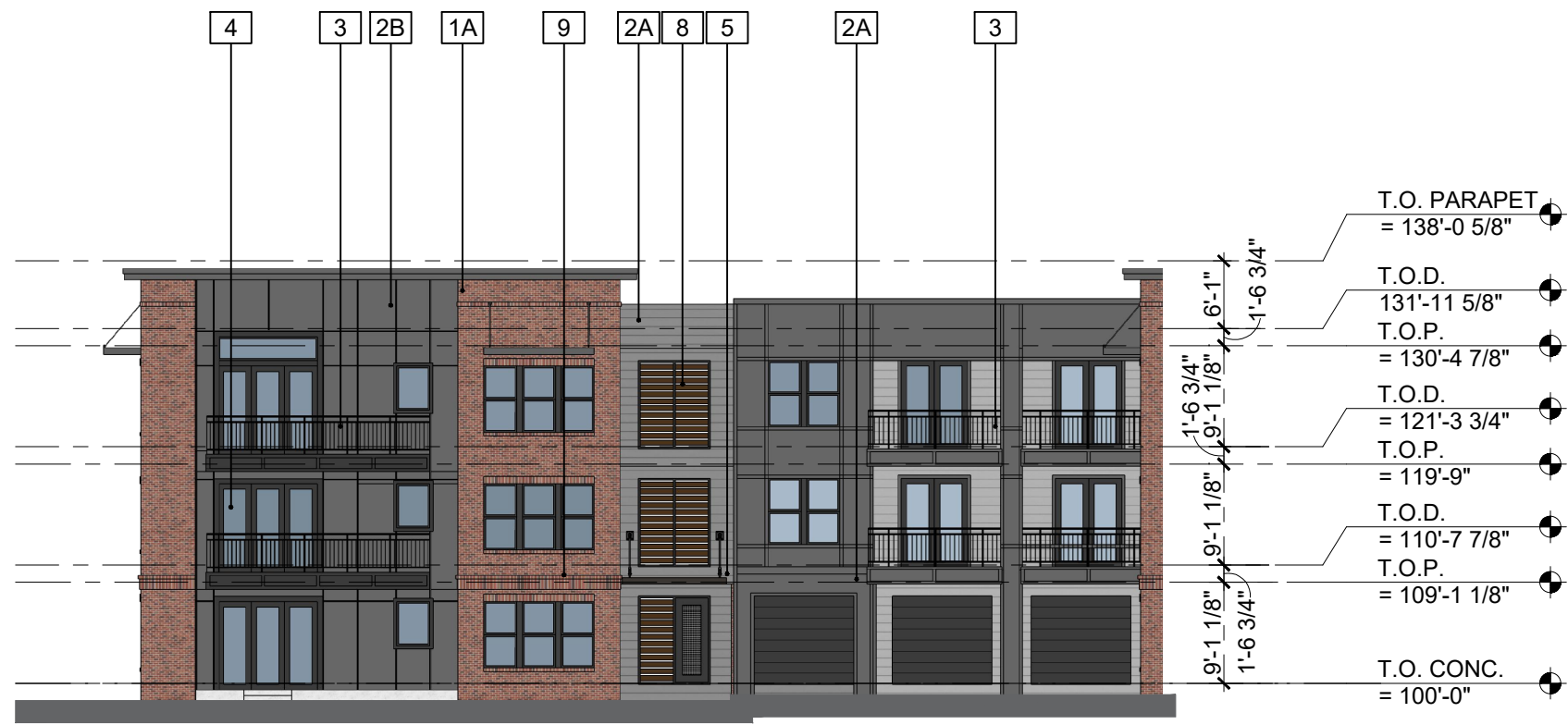
03 BLDG #2 & 3 - EAST ELEVATION SCALE: 1/16" = 1'-0"
