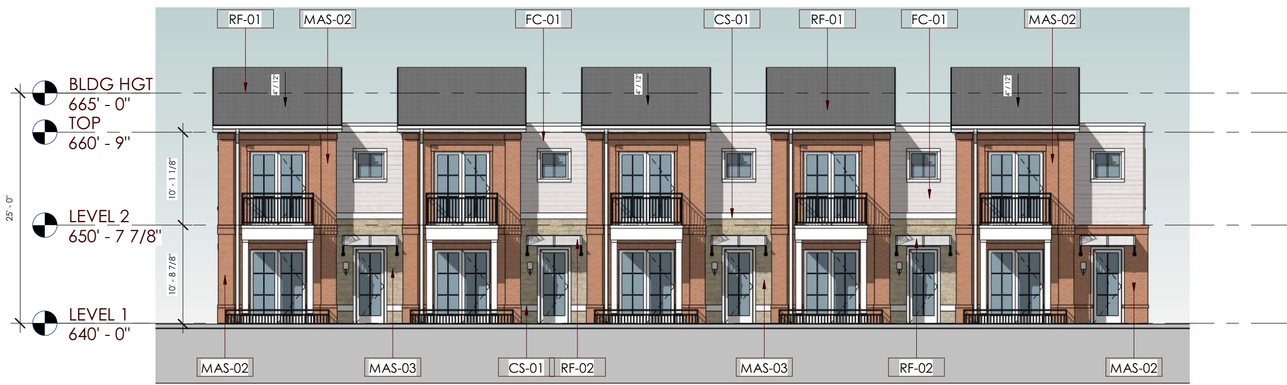
1 BUILDING C1/C4 - FRONT ELEVATION SCALE: 3/32" = 1'-0" BRICK = 59% STONE = 22% C1/C4 TOTAL BRICK = 70.5% STONE = 7.5% FIBER CEMENT = 19% FIBER CEMENT = 22% GLASS = 19% GLASS = 13%
