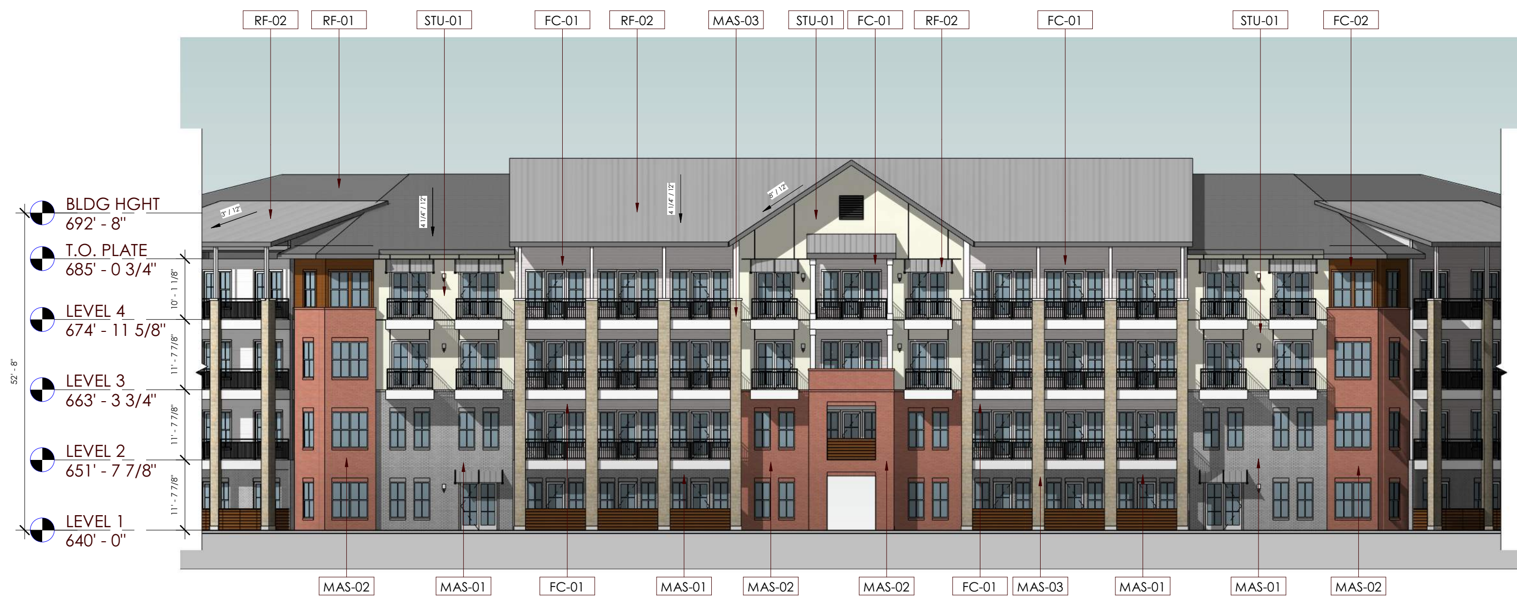
1 BUILDING B - SOUTH ELEVATION SCALE: 1/16" = 1'-0"
