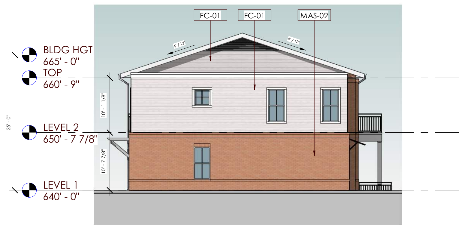
5 BUILDING C - SIDE ELEVATION - B SCALE: 3/32" = 1'-0" BRICK = 51% STONE = 0% FIBER CEMENT = 49% GLASS = 7%
