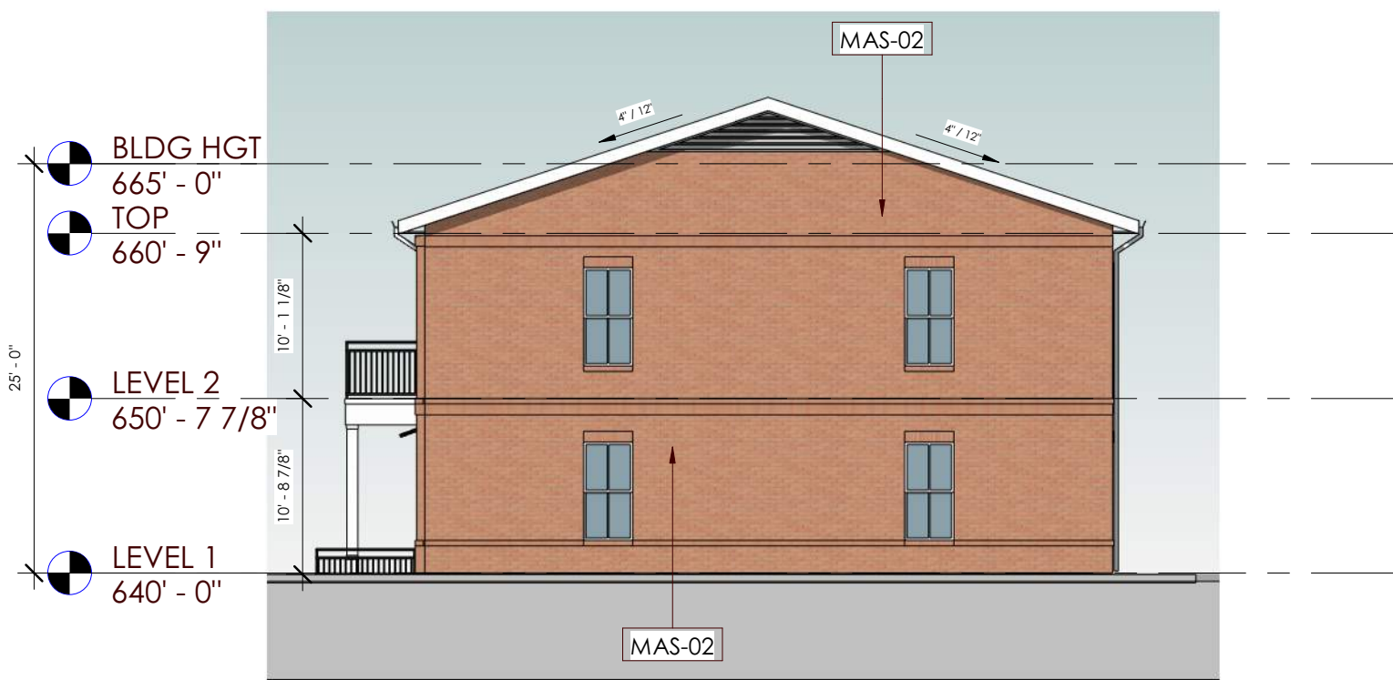
7 BUILDING C - SIDE ELEVATION - A SCALE: 3/32" = 1'-0" BRICK = 100% STONE = 0% FIBER CEMENT = 0% GLASS = 8%
