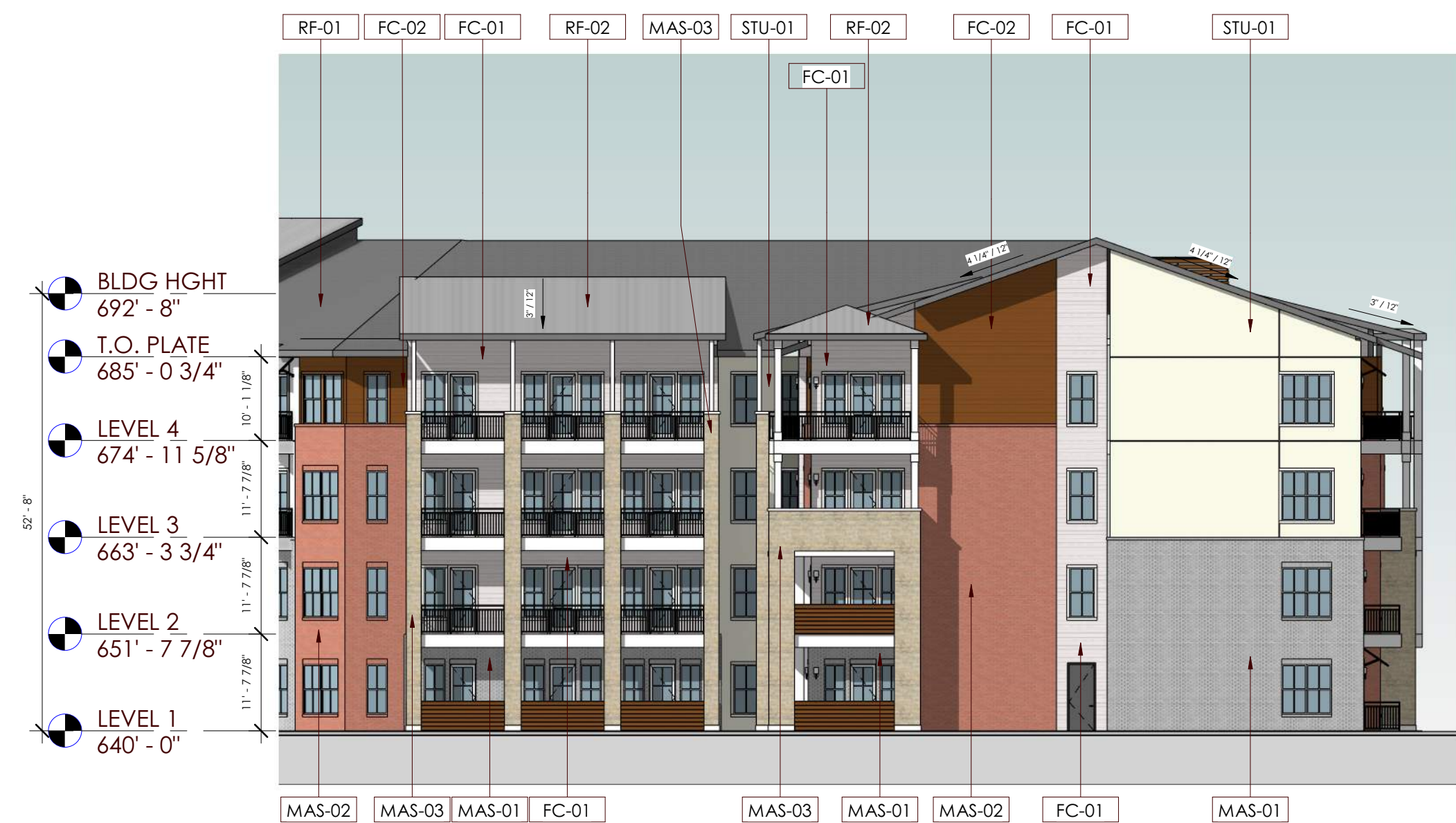
2 BUILDING B - SE WING ELEVATION SCALE: 1/16" = 1'-0"
