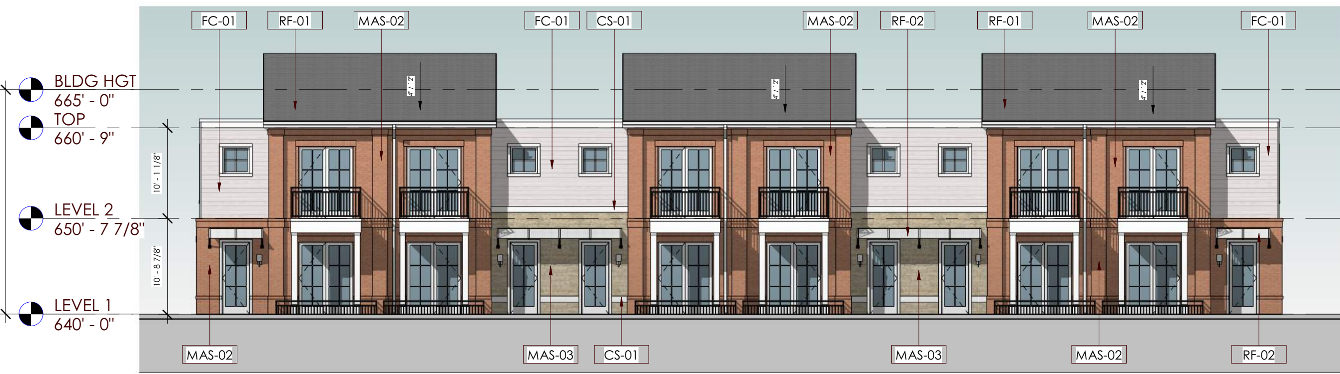
3 BUILDING C5 - FRONT ELEVATION SCALE: 3/32" = 1'-0" BRICK = 59% STONE = 22% C5 TOTAL BRICK = 62% STONE = 8% FIBER CEMENT = 19% FIBER CEMENT = 30% GLASS = 19% GLASS = 13%
