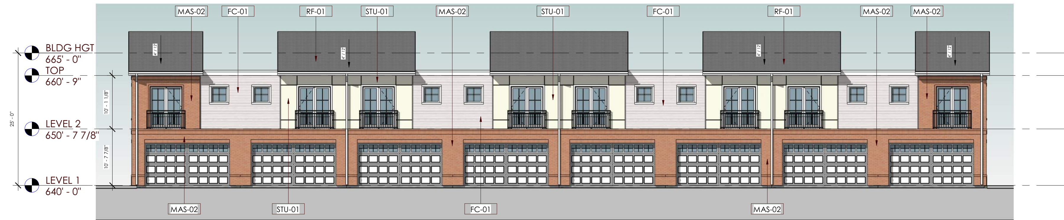
8 BUILDING C2/C3 - REAR ELEVATION SCALE: 3/32" = 1'-0" BRICK = 77% STONE = 0% FIBER CEMENT = 23% GLASS = 11%
