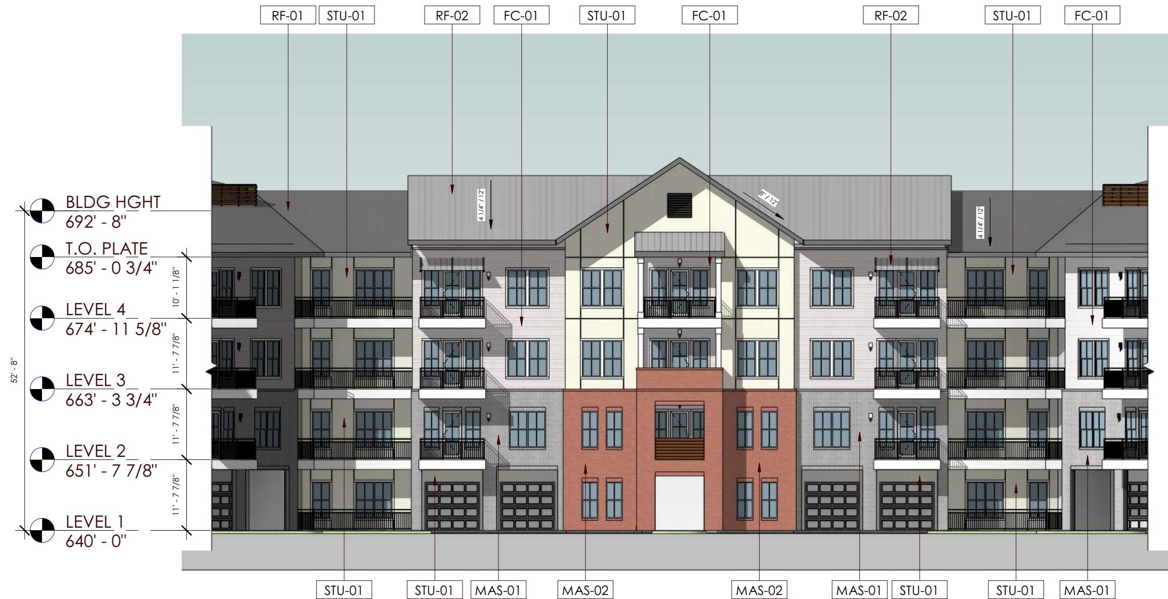
6 BUILDING B - NORTH ELEVATION SCALE: 1/16" = 1'-0"
