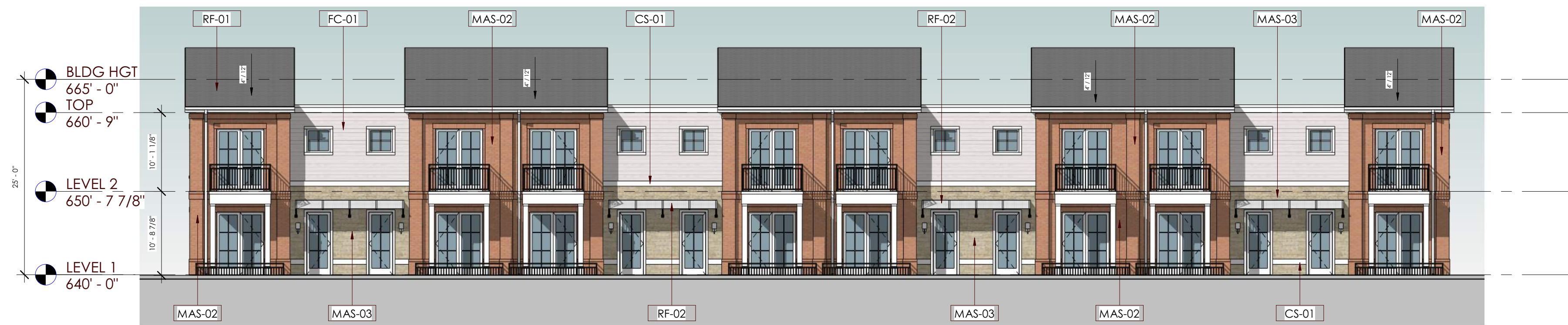
6 BUILDING C2/C3 - FRONT ELEVATION SCALE: 3/32" = 1'-0" BRICK = 59% STONE = 22% C2/C3 TOTAL BRICK = 76.5% STONE = 8.5% FIBER CEMENT = 19% FIBER CEMENT = 15% GLASS = 19% GLASS = 14%
