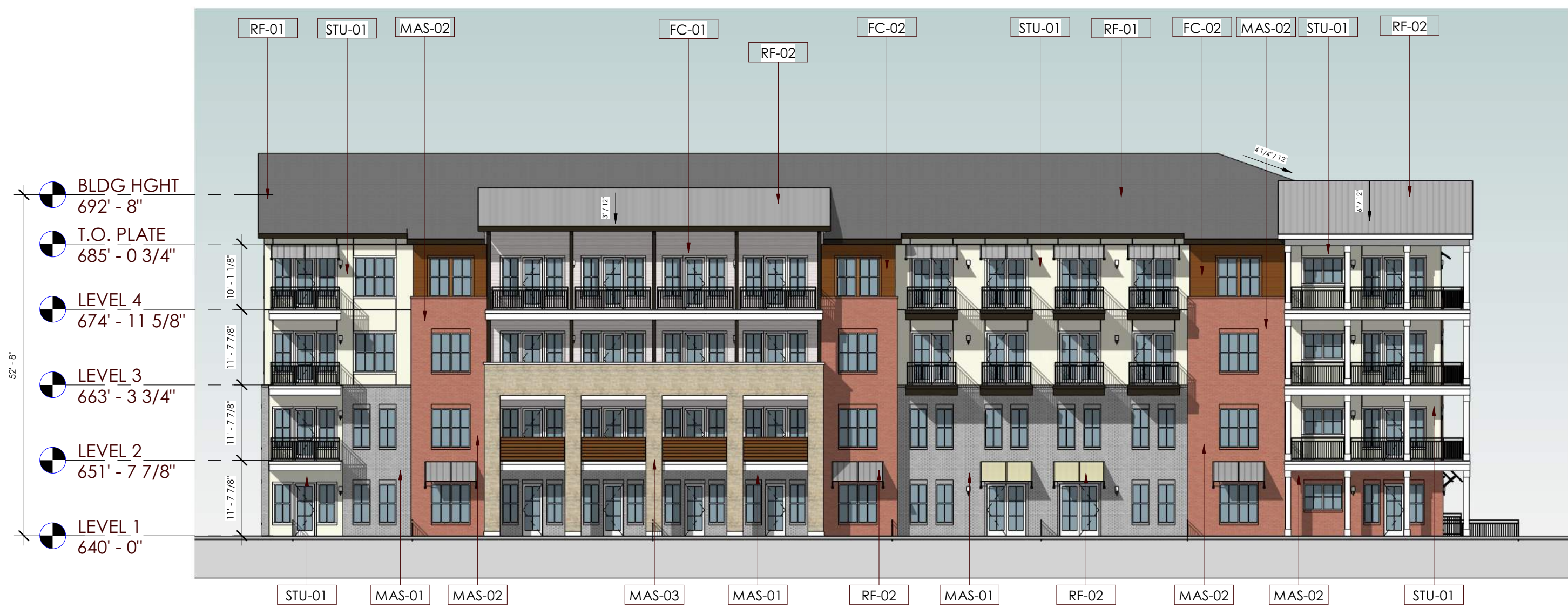
3 BUILDING A - WEST ELEVATION (EAST O.H.) SCALE: 1/16" = 1'-0"
