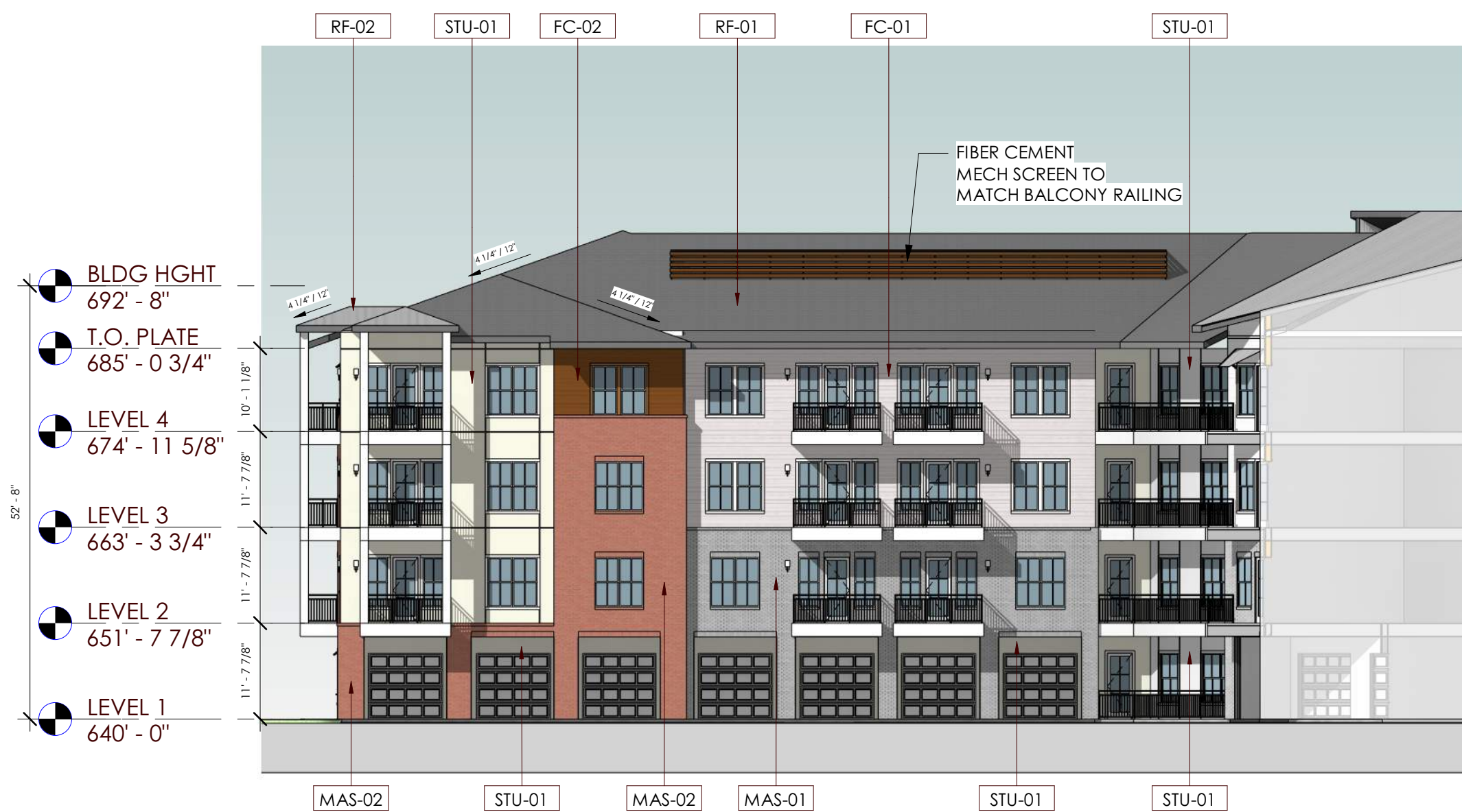
5 BUILDING B - NW WING ELEVATION SCALE: 1/16" = 1'-0"
