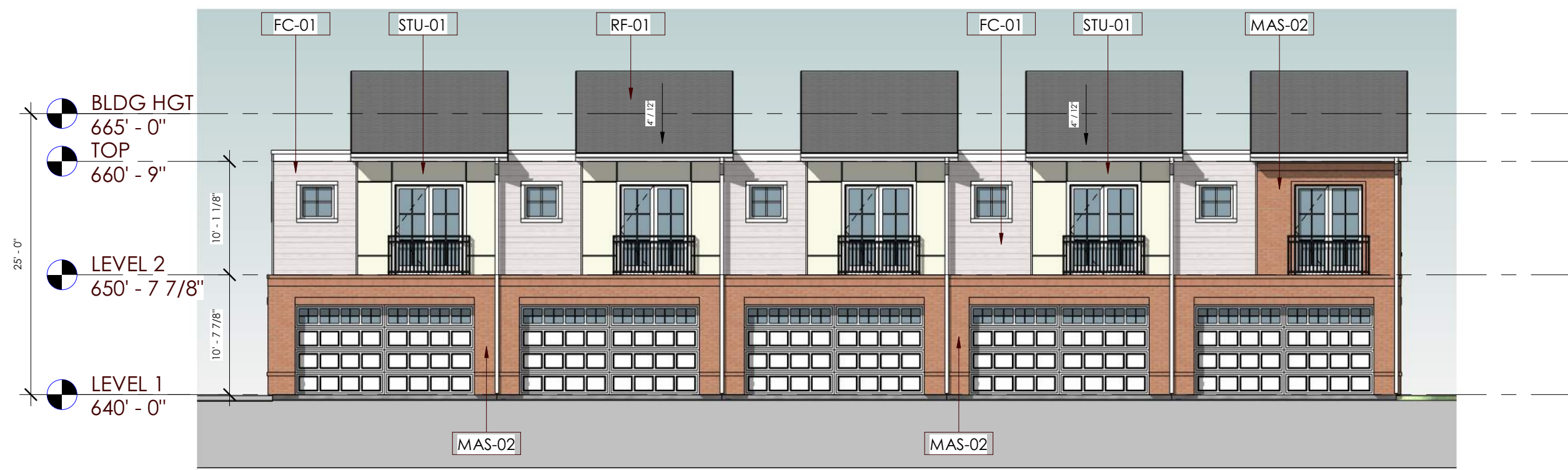
2 BUILDING C1/C4 - REAR ELEVATION SCALE: 3/32" = 1'-0" BRICK = 77% STONE = 0% FIBER CEMENT = 23% GLASS = 11%
