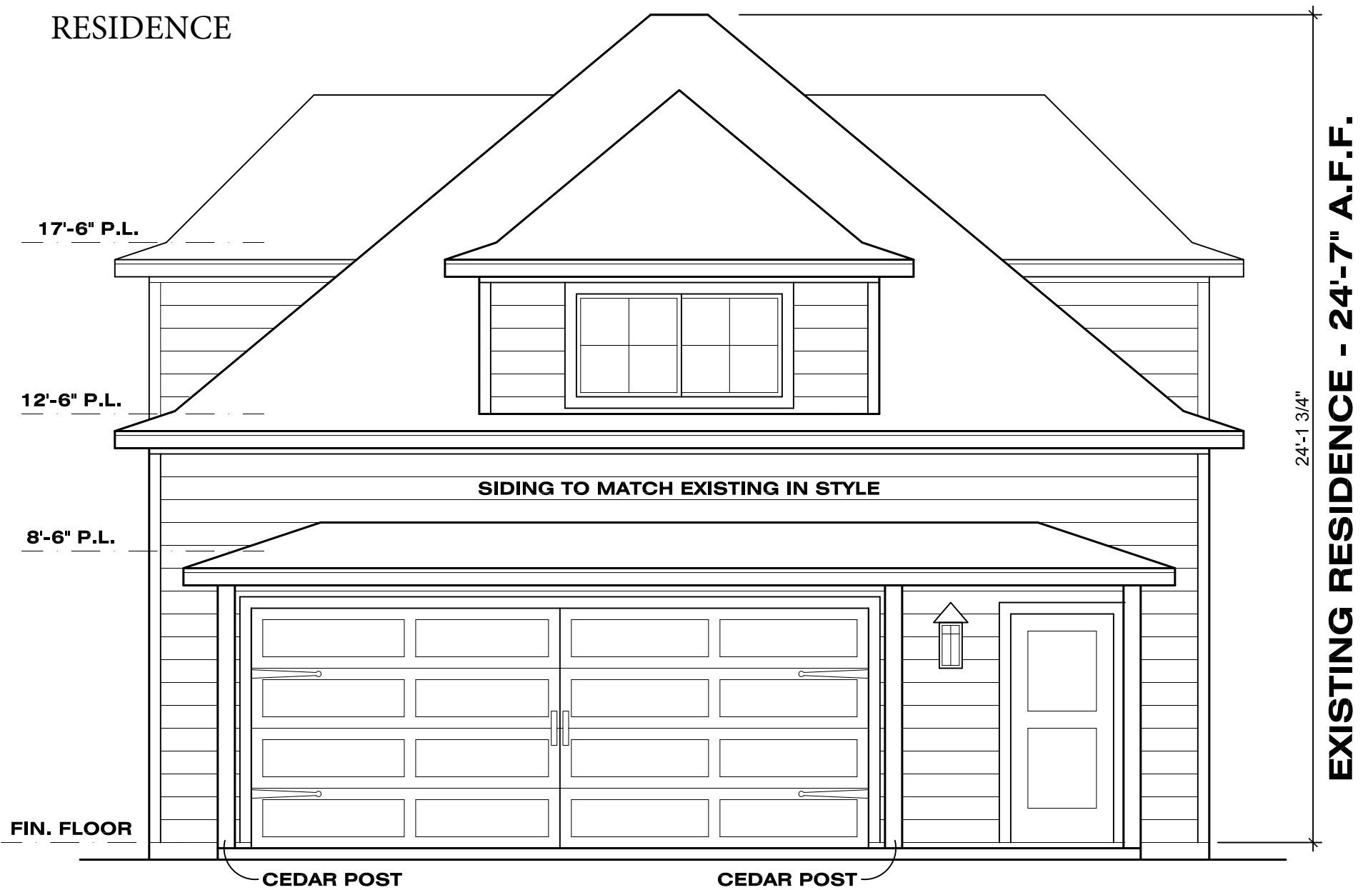
FRONT ELEVATION SCALE:1/4"=1'-0" CEMENTITIOUS SIDING AND TRIM, TYP.
