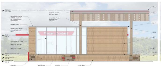
T.O. ROOF 119' - 7 3/4" BRICK VENEER. (M-1) STONE WATER TABLE (M-3) (M-3) STONE WAINSCOT M-2 BOLLARD
