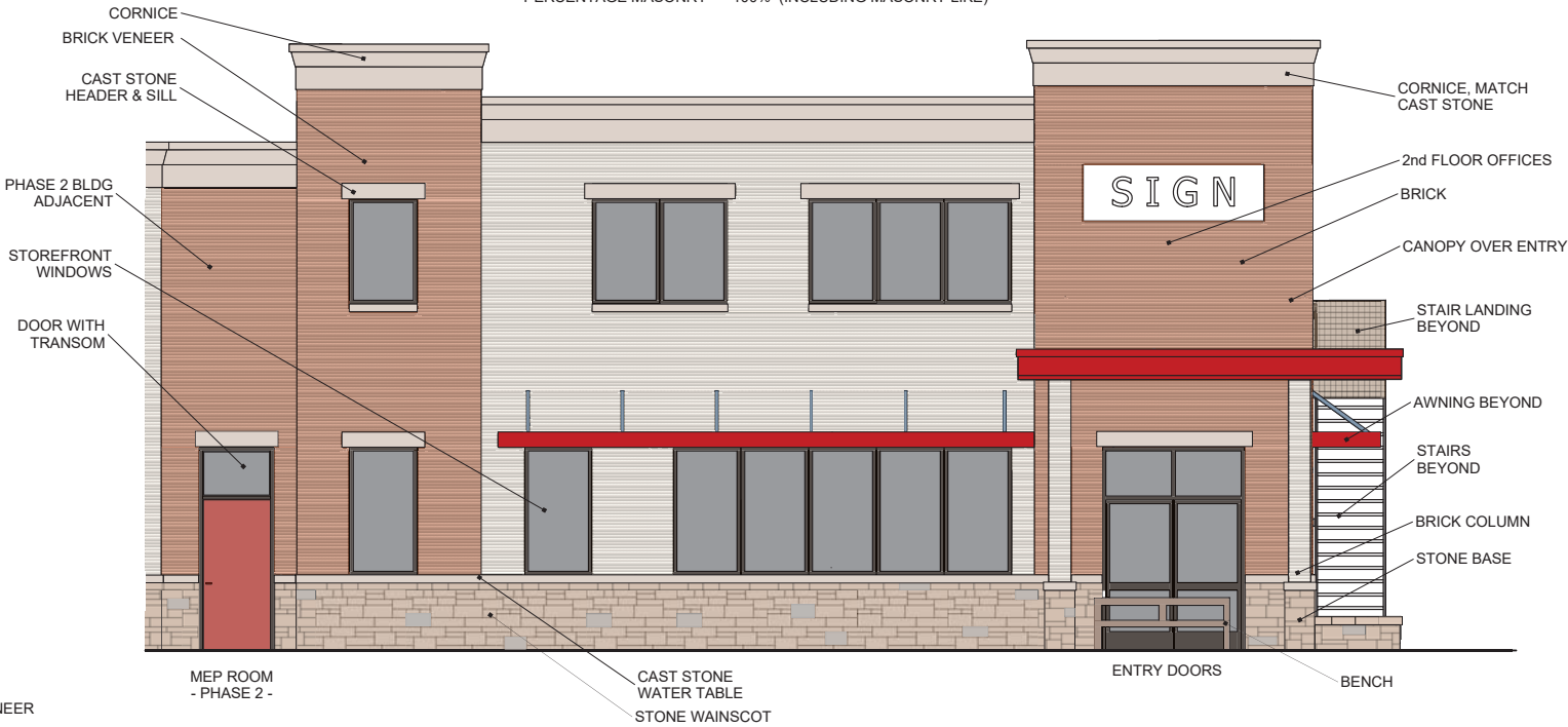
SOUTH FRONT ELEVATION: TURNER WARNELL SIDE WALL MATERIALS: MASONRY (BRICK & STONE) = 802.5 SQUARE FEET CORNICE (MASONRY LIKE) = 90.0 SQUARE FEET PERCENTAGE MASONRY = 96.8% (EXCLUDING WINDOWS, DOORS & AWNINGS) SCALE: 1/4" = 1'-0"
