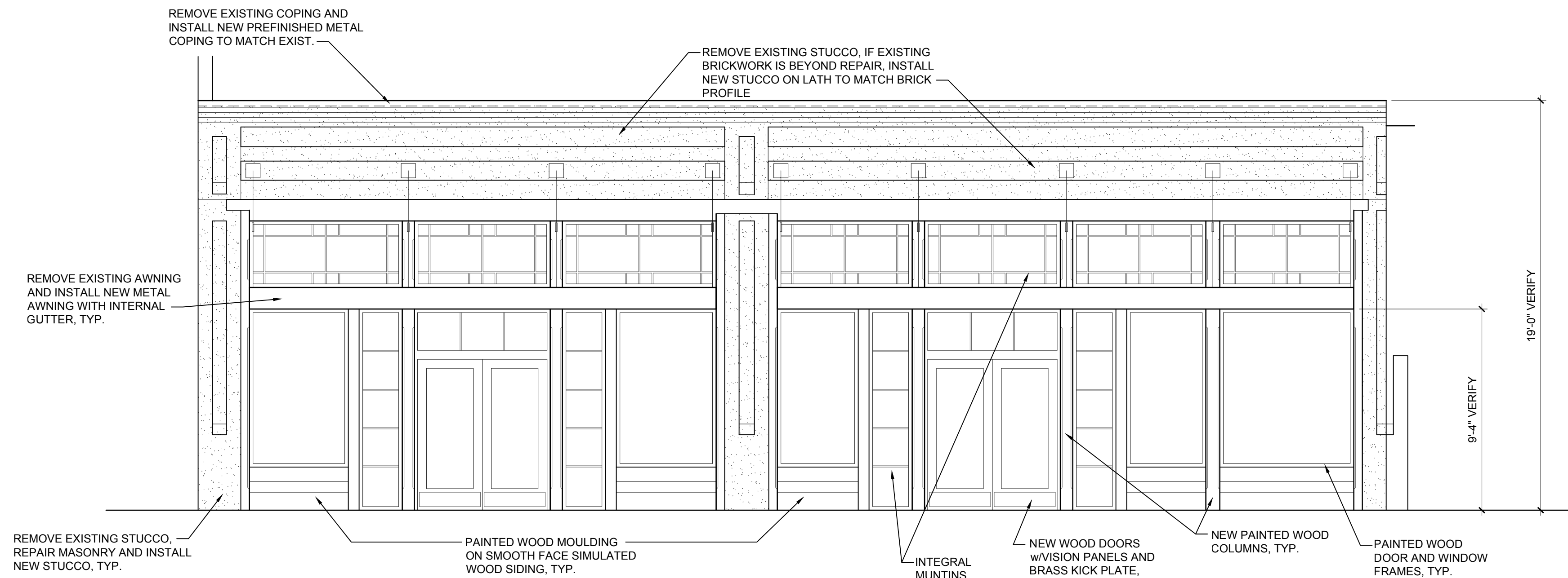
2 REVISED EAST ELEVATION - OPTION 2 SCALE: 1/4" = 1'-0"
